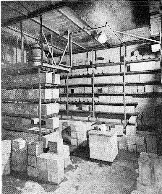
Photo 3. Climate room:  $\varphi = 95 \dots 100 \%$ ,  $t = 20^\circ\text{C}$ ,  $v < 0.5 \text{ m/s}$ . Demoulding and/or crushing of the specimens was effected here.
