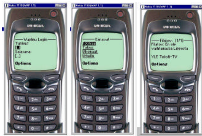
Figure 5. The WAP-IMU publication, where the user at first logs in, selects a channel (Kotimaa), a heading and finally gets a short article.
