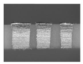
Figure 7: Sintered and Diced Via Plugs with Diameter of 0.4 mm, 0.3 mm and 0.25 mm. Substrate thickness is 0.5 mm.
