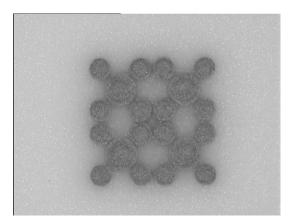
Figure 5: Thermal Via Structure for 2×2 LED Array on 0.5-mm Thick Alumina Substrate. Via diameters are 0.4 mm and 0.25 mm.
