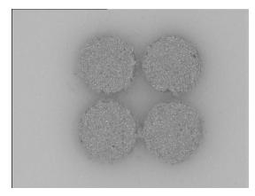
Figure 6: Thermal Via Structure for  $2 \times 2$  LED Array on 0.63 mm Thick Alumina Substrate. Via Diameter is 0.9 mm.
