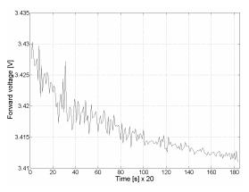
Figure 11: Forward Voltage of Blue LED on 1 mm Thick Alumina Substrate.
