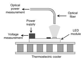
Figure 9: Measurement Setup for LED Modules.
