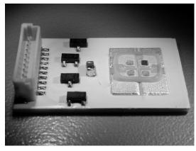
Figure 8: Prototype LED Module.
