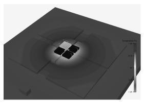
Figure 4: Simulated Surface Temperatures of Prototype Module with 1-mm Thick Substrate.
