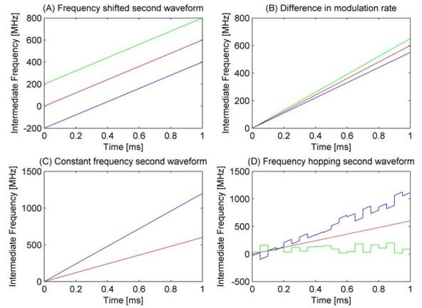
Figure 2. Different harmonic waveforms (in the intermediate frequency band). Base signal 1 and 2 are in red and green respectively. The transponder return signal is in blue.
