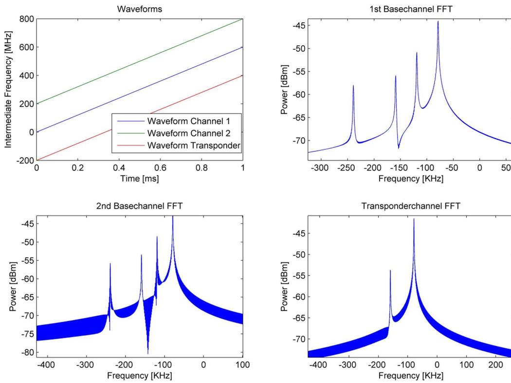
Figure 4. Simulation results of dual channel radar architecture.
