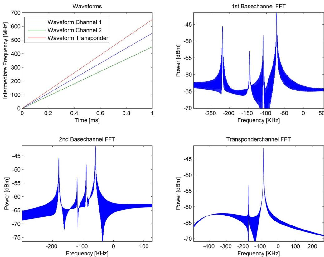
Figure 5. Simulation results of the single channel radar architecture.
