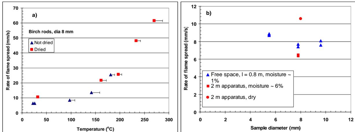
**Figure 4** a) rate of flame spread on 8 mm birch rod samples, b) comparison between flame spread rate on birch rods measured in free space and in the 2 m apparatus
