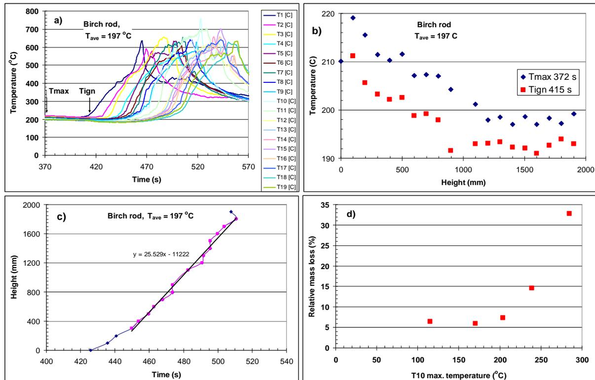
**Figure 3** Flame spread on a cylindrical birch sample. a) temperature-time curves,  $T_{max}$  and  $T_{ign}$  indicated with arrows, b) vertical temperature distribution at times for  $T_{max}$  and  $T_{ign}$ , c) straight line fit to height – time plot, criterion: time when  $T > 300\text{ °C}$ , d) relative mass loss including moisture from reference birch samples
