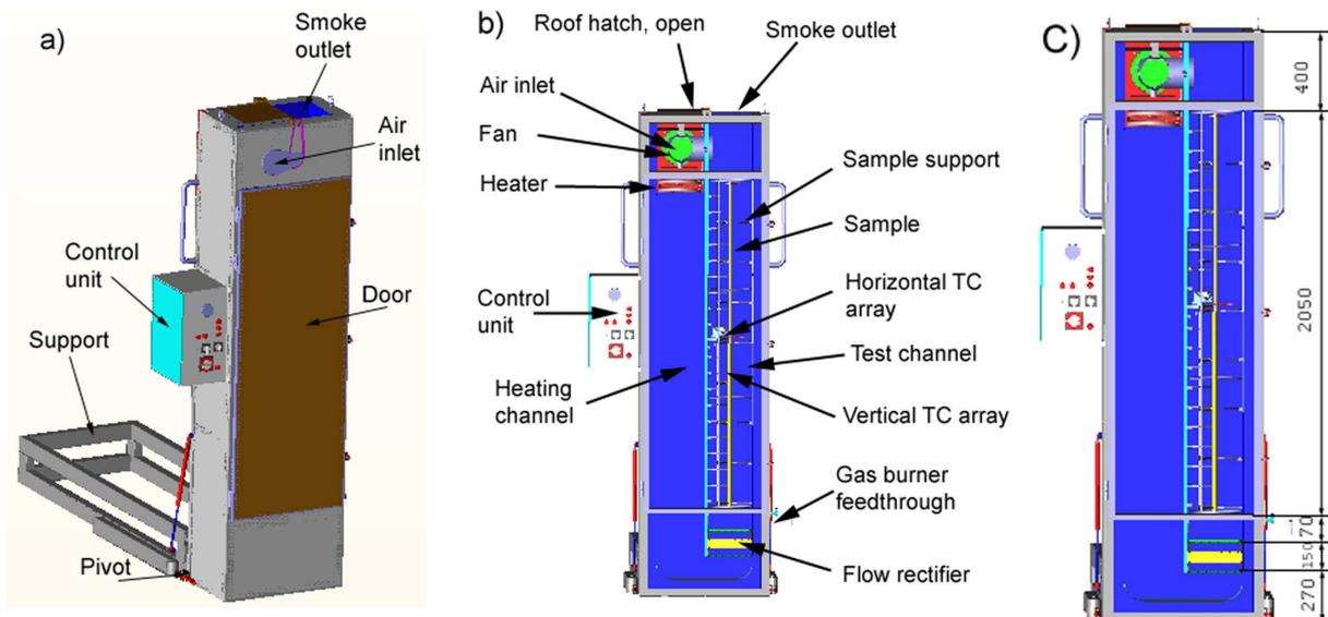
**Figure 1** 2 m test rig in vertical position; a) general view, b) cross-section with essential features, c) vertical dimensions in mm
