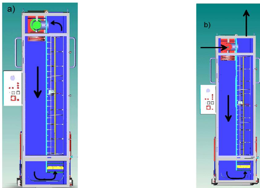
**Figure 2** a) circulation of air during heating phase, b) fresh air intake to heating channel and fire effluent outlet from top of test channel during experiment, upper opening connecting the channels closed
