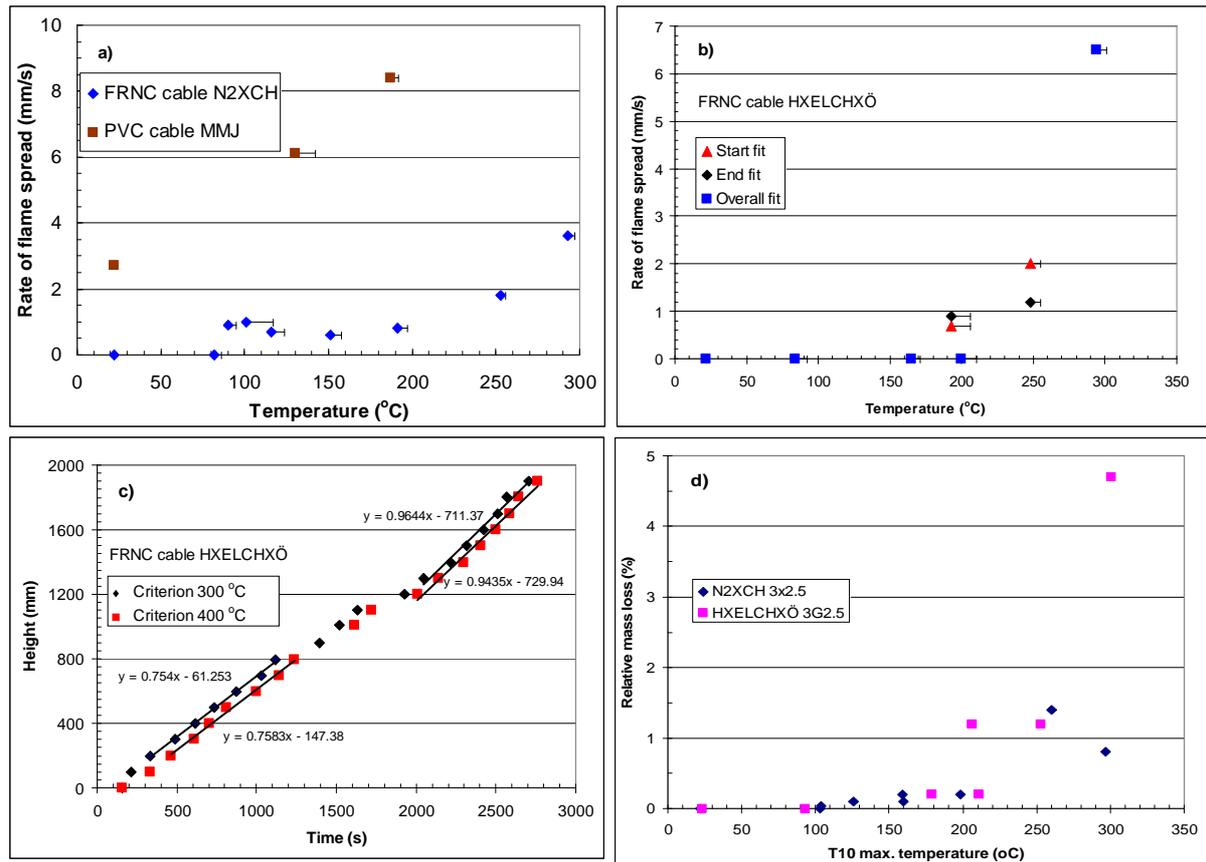
**Figure 5** a) and b) rate of flame spread on PVC and FRNC cables, c) uniformity of rate of flame spread determined with two temperature criteria, separately for start and end of experiment, d) reference sample loss in FRNC cable experiments
