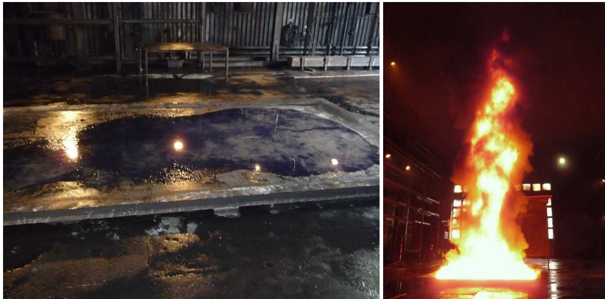
Figure 3 Left: the concrete pad with a pre-spill of 60 l of turbine oil; right: the test fire without the steel table. The maximum flame height is about 8 m
