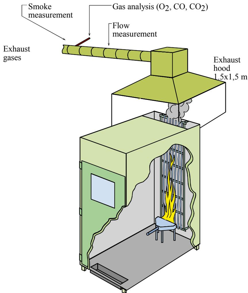
Figure 5. Cable test equipment according to EN 50266.
