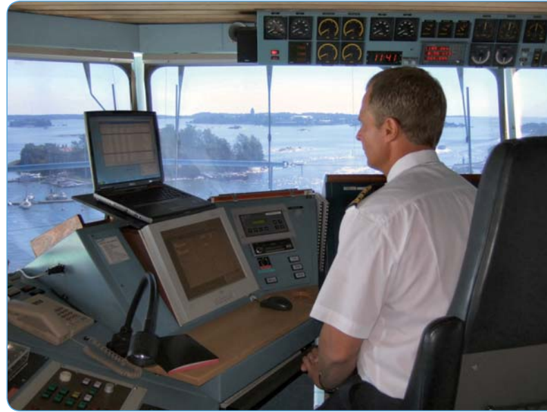
Figure 2. The field tests were realised by connecting a laptop computer to the onboard AIS equipment.
