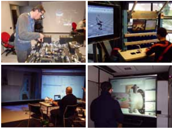
Figure 5. The first tool (top left) provides real time contextualized work instructions with the use of AR. The second tool (top right) implements a real time physical ergonomic analysis with a motion capture system and it also allows an ergonomic specialist to handle the evaluation process. The third tool (bottom left) supports task planning and procedure validation in a VE by the designers and ergonomic specialists. The resulting tasks can be fed into the first tool for the instruction delivery. The fourth tool (bottom right) utilises a haptic device in a VE to support motor skill training in accordance with the precision teaching method
