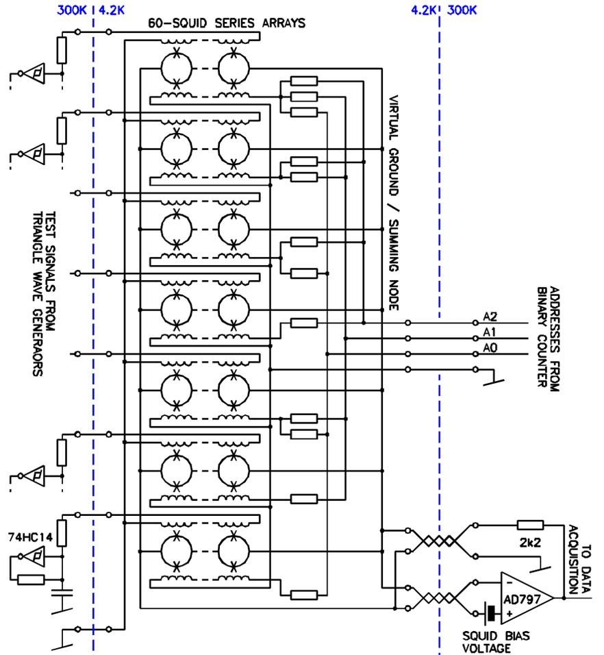
Fig. 4. Simplified schematic of the experimental setup.
