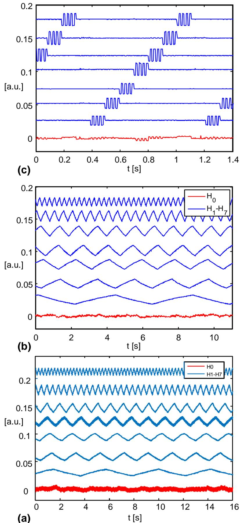
Fig. 5. Encoded, digitized and decoded test signals: triangle wave signals encoded (a) at 3900 frames per second and (b) at 310 frames per second, and (c) two-level calibration bursts encoded at 310 frames per second. Arbitrary units are used in the vertical axis. There is no SQUID-encoded signal in the H<sub>0</sub> channel although it is decoded and included in the plots. Decoding was performed by the ideal Hadamard matrix rather than by inverse of the true encoding matrix.
