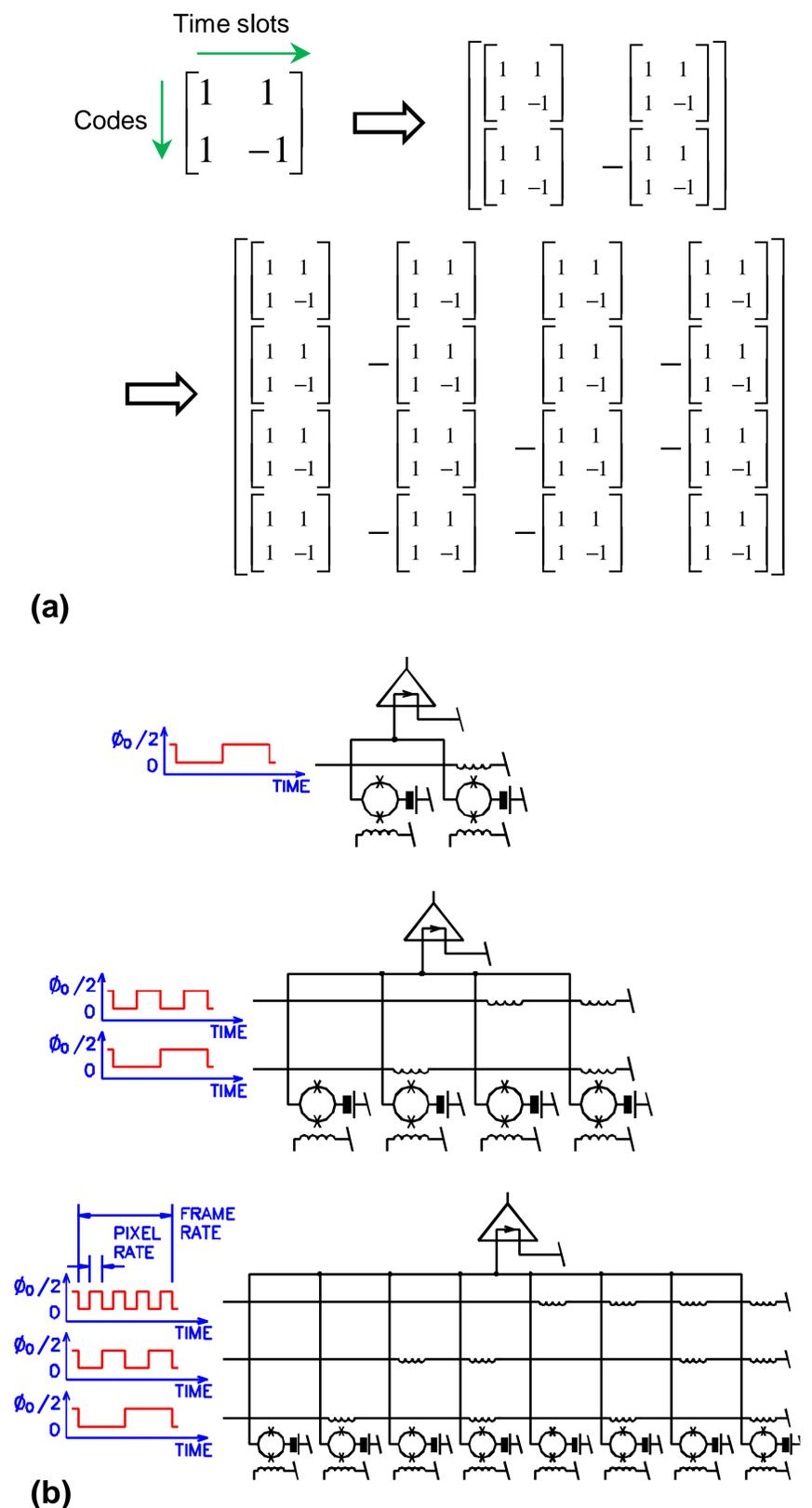
Fig. 3. (a) Hadamard matrices can be generated by taking the primitive  $2 \times 2$  matrix and by recursively replacing its elements with copies of the primitive matrix. In the multiplexing context the rows correspond to signal channels and columns correspond to time slots. (b) The recursive procedure is equivalent to repeated doubling of the primitive 2-SQUID cell when an additional double-rate  $\Phi_0/2$  flux shift is summed to the lower half of the new cell.
