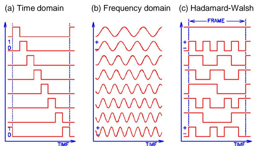
Fig. 1. Three orthogonal basis sets generally used for cryogenic multiplexing.
