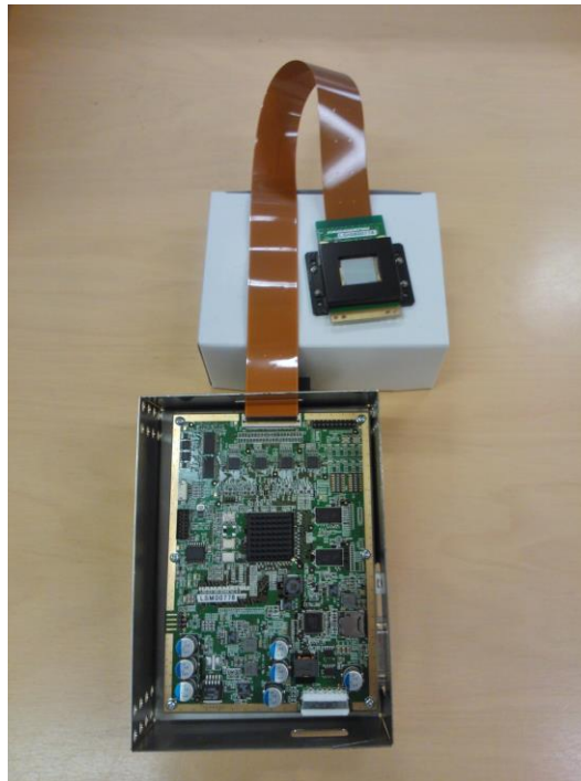
Fig. 4.1.1 Hamamatsu OEM Lcos-SLM X11840-03 display and controlling unit with the self-build cover.
