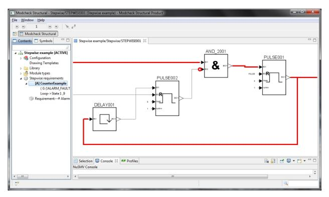
Fig 2. In VTT's tools, function block diagrams are modelled with a graphical UI. The model is transformed into the input language of NuSMV, the model checker is run, and the counterexamples are visualised with an animation.
