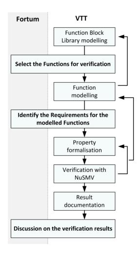
Fig 1. The work process for model checking in LARA
