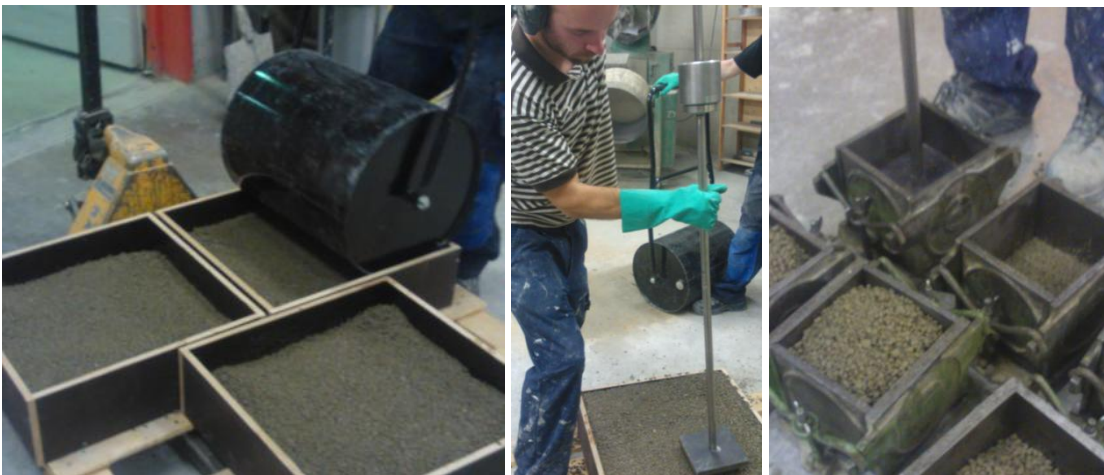
Figure 3 – PC-slab and specimen casting and compaction.
