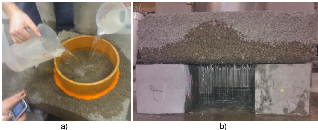
Figure 8 – PC-slab water infiltration measurements showing high water infiltration rate: a) ASTM single ring method for PC; b) ASTM double ring method (for soil).
