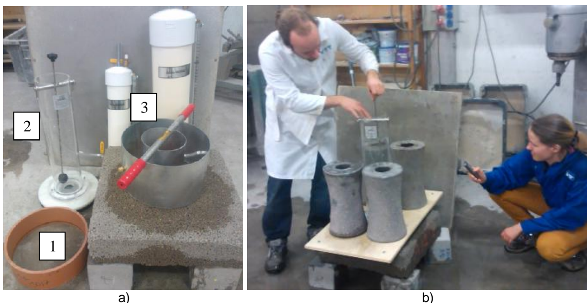
Figure 5 – Water infiltration testing. a) Testing equipment for 1) ASTM C1701, 2) EN 12697-40 and 3) ASTM D3385; b) Testing by EN 12697-40 (falling head permeameter for asphalt in situ drainability).
