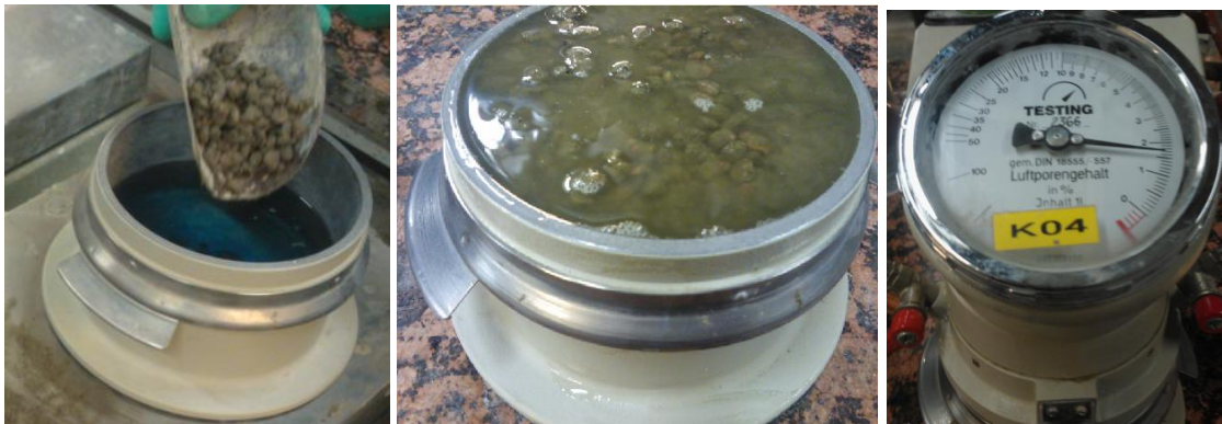
Figure 4 –Test method for entrained air content of freshly mixed PC by a tentative ‘modified pressure method’. Interconnected voids are excluded.
