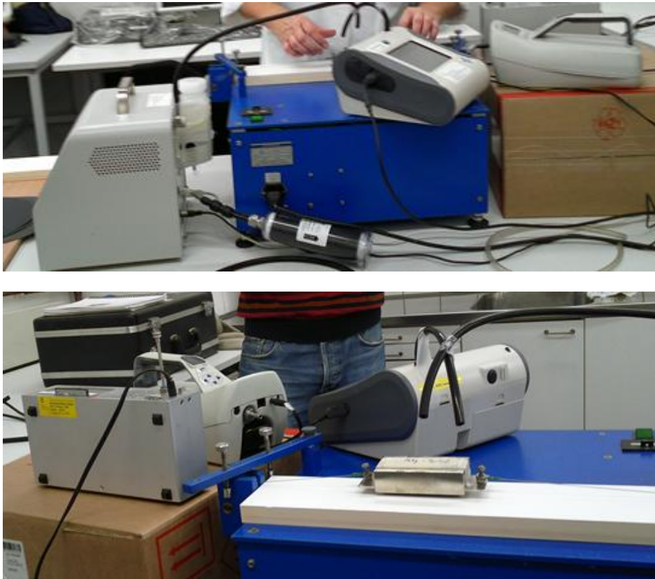
Figure 4. The instrumentation for particle emissions during the abrasion tests.
