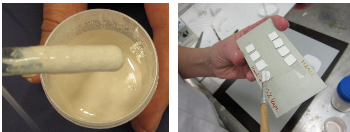
Figure 18. (a) PS-IPDI microcapsules mixed into polyester paint and (b) Polyester paints with and without PS-IPDI microcapsules.
