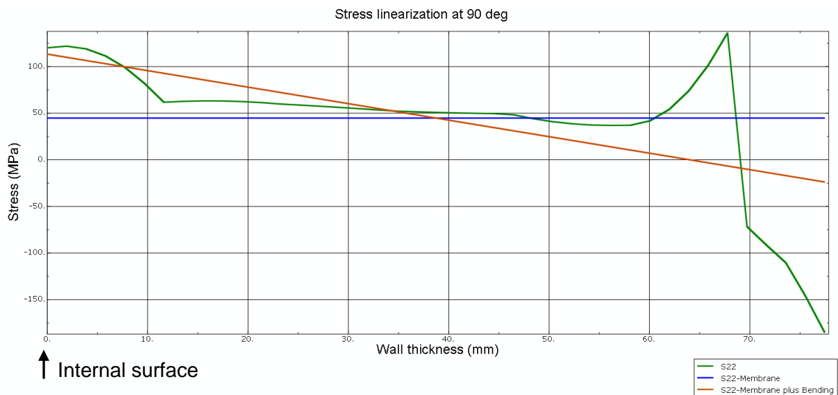
Figure 13. The stress linearization for the axial stress component (S22). Blue line indicates the membrane stress and the orange line indicates the combined membrane+bending stress.
