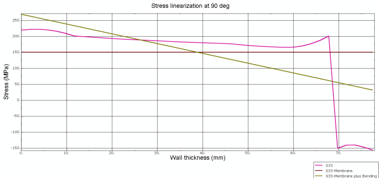
Figure 19. The stress linearization for the circumferential stress component ( S_{33} ). Brown line indicates the membrane stress and the green line indicates the combined membrane+bending stress.
