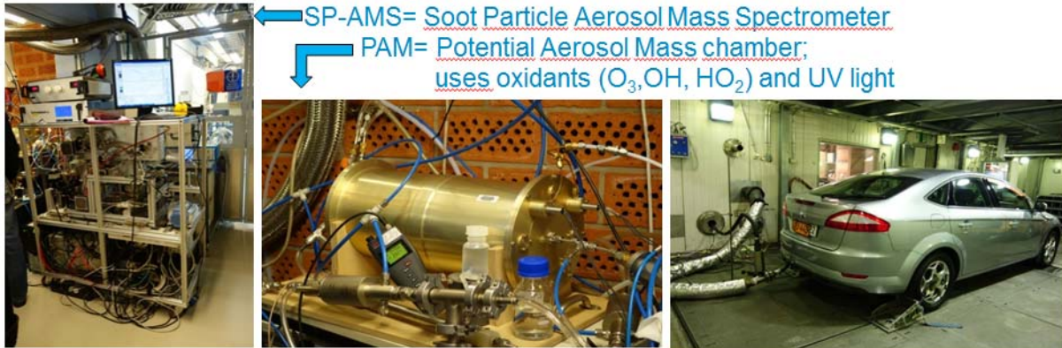
Figure 2. FMI characterized before and after PAM from sub-micron PM: organics, sulfate, nitrate, ammonium, chloride, black carbon and metals.
