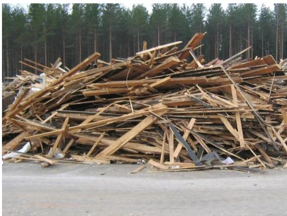
**Figure 6.** Example of class C wood, demolition wood. Photo VTT.
