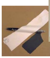
Electrospun PAN and carbonized sheet
