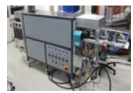
Stabilization (<300°C) and carbonization (<1500°C) at R2R oven.
