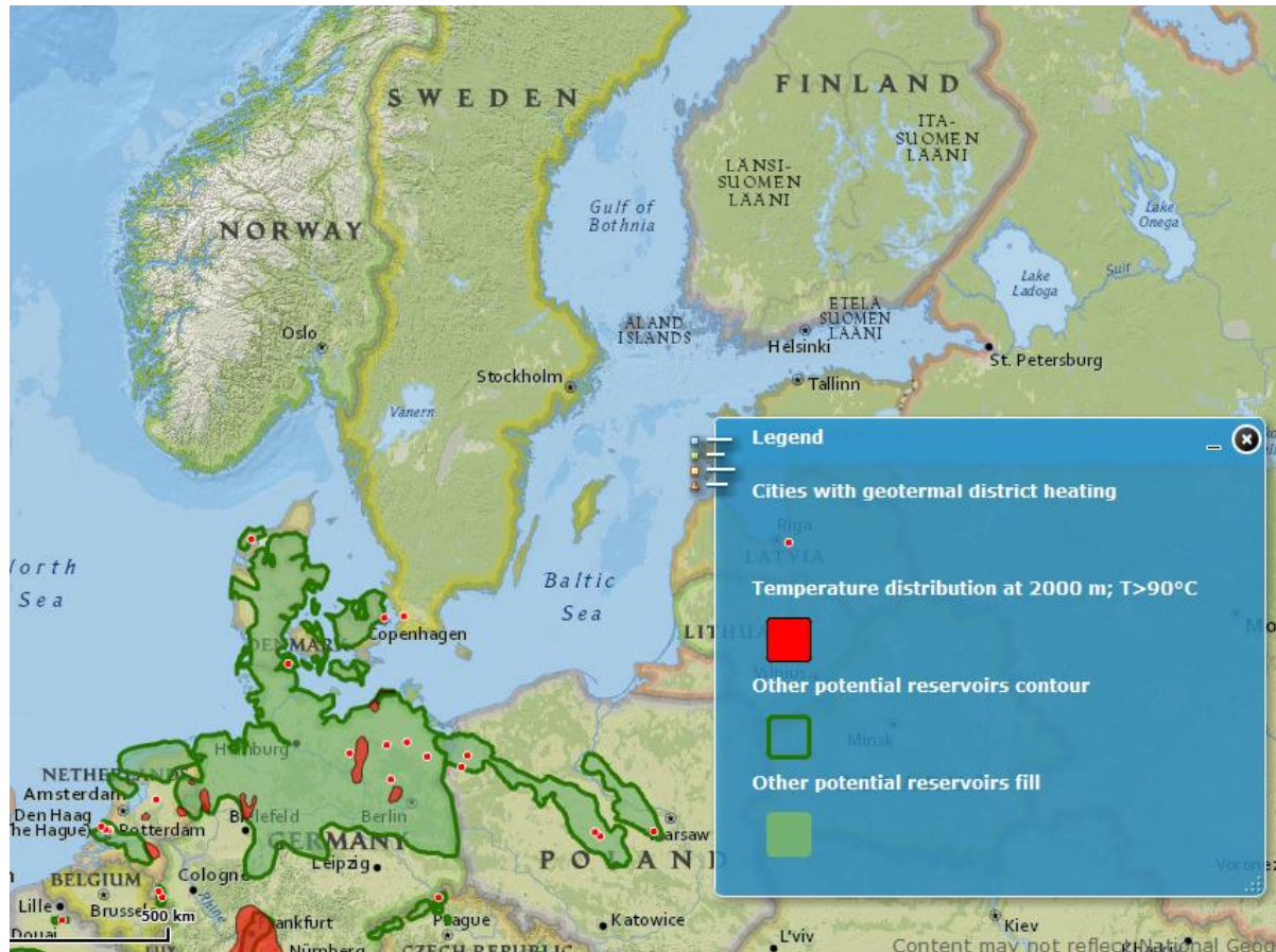
Figure 8. Deep geothermal heat sources according to EU project Geo DH Europe (GeoDH 2013, 2014a). Red areas have temperatures above 90 °C at 2 000 m depth and green areas have other reservoir potentials. Red spots indicate DH networks using geothermal heat. Source: Interactive map at http://loczy.mfgi.hu/flexviewer/geo_dh/
