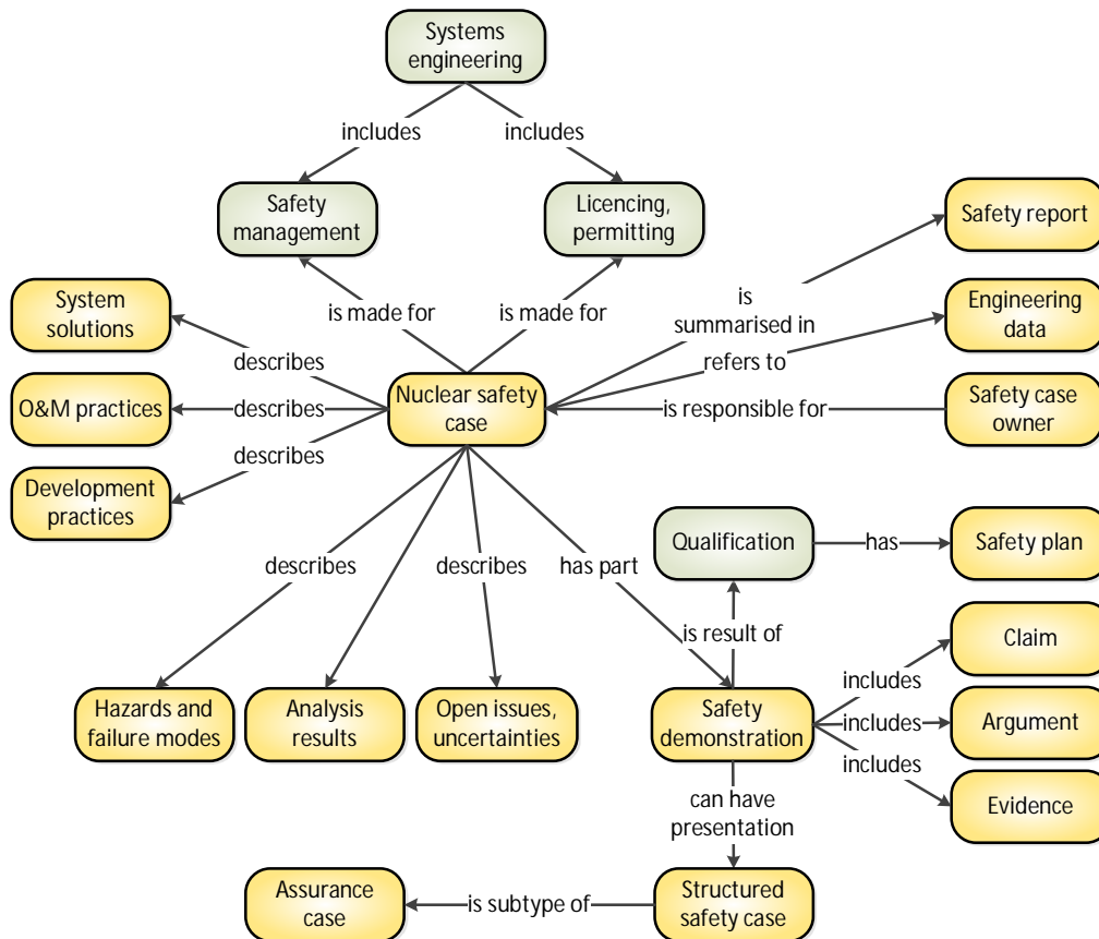
Figure 2. Key concepts related to a nuclear safety case. Artefacts are shown as yellow and processes as green boxes.
