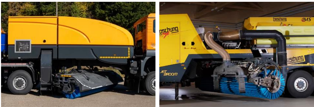
Figure 6. Limited space for broom in Aebi Schmidt (left picture) and Boschung
