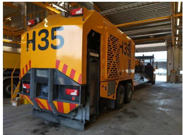
Figure 4. A PSB's blower (blower arm not deployed)
