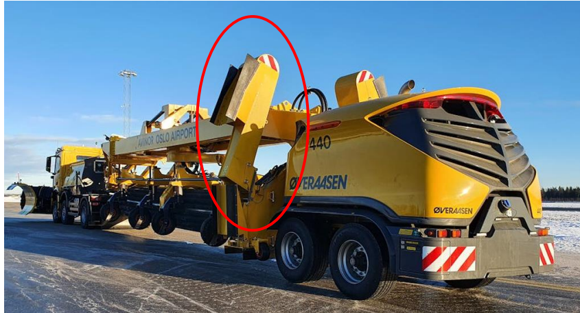
Figure 7. Øveraasen RS 600 with blower nozzles pulled to the sides.
