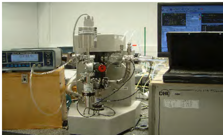
Fig. 2. The transfer standard (on the left) and the reference standard of MIKES
