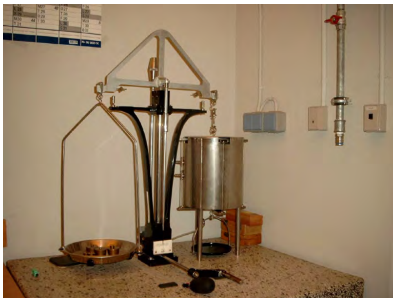
Fig.9. The low gauge pressure standard of FORCE Technology.
