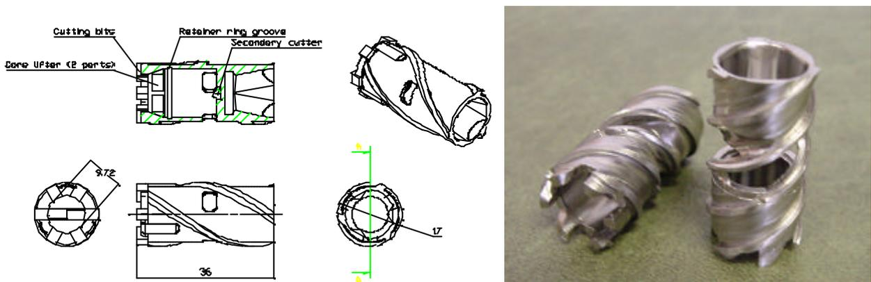
**Figure 11. Tool design and prototypes (missing drill bits here).**
