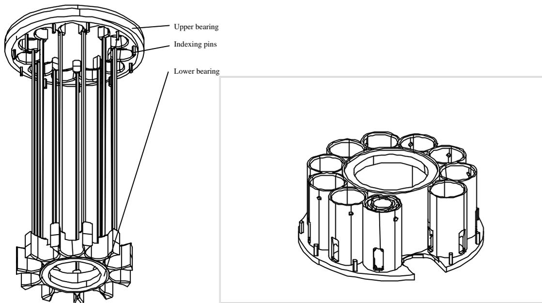
**Figure 9. Pipe carousel and tool carousel.**
