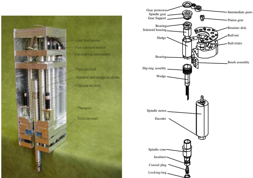
**Figure 3. DSS and an exploded view of the spindle.**
