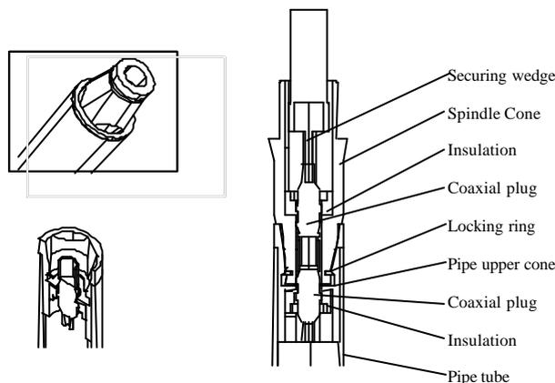
**Figure 4. Design of the coupling.**
