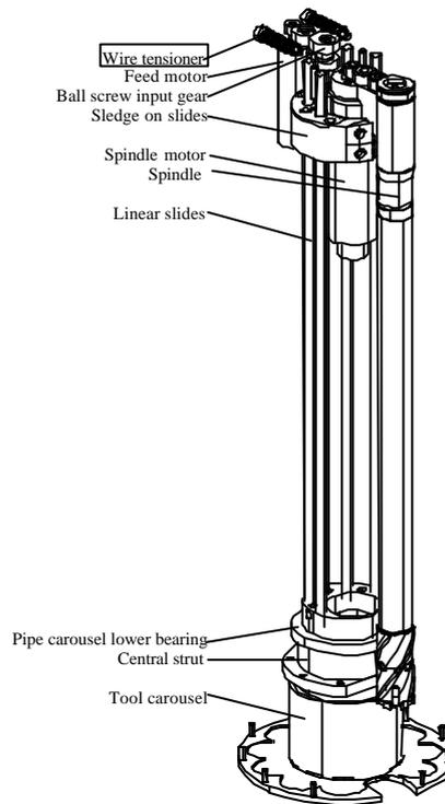
**Figure 8. Linear feed system.**
