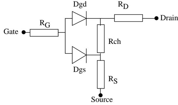
**Figure 1** DC equivalent circuit of MESFET for cold-FET ( $V_{ds}=0$ ) applications.
