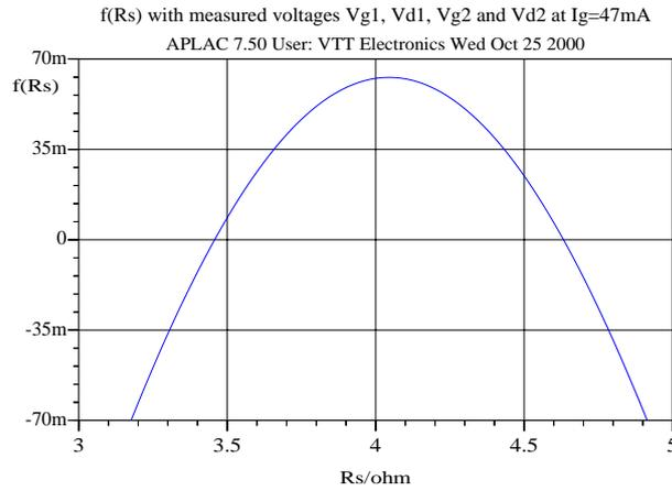
**Figure 2** Function  $f(R_s)$  of a MESFET with measured voltages  $V_{g1}$ ,  $V_{d1}$ ,  $V_{g2}$  and  $V_{d2}$  at  $I_g=47mA$ .
