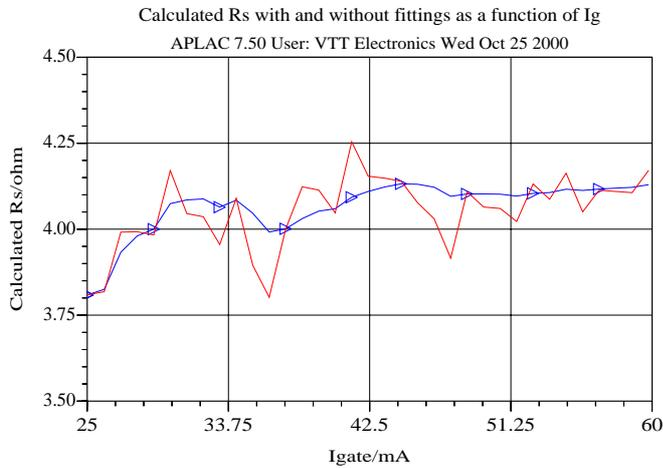
**Figure 3** Analytically solved  $R_S$  as a function of  $I_g$  with and without function fittings.
