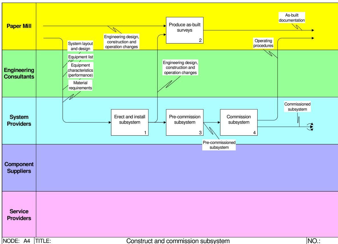
Figure 10. Construct and commission changes in the paper mill.
