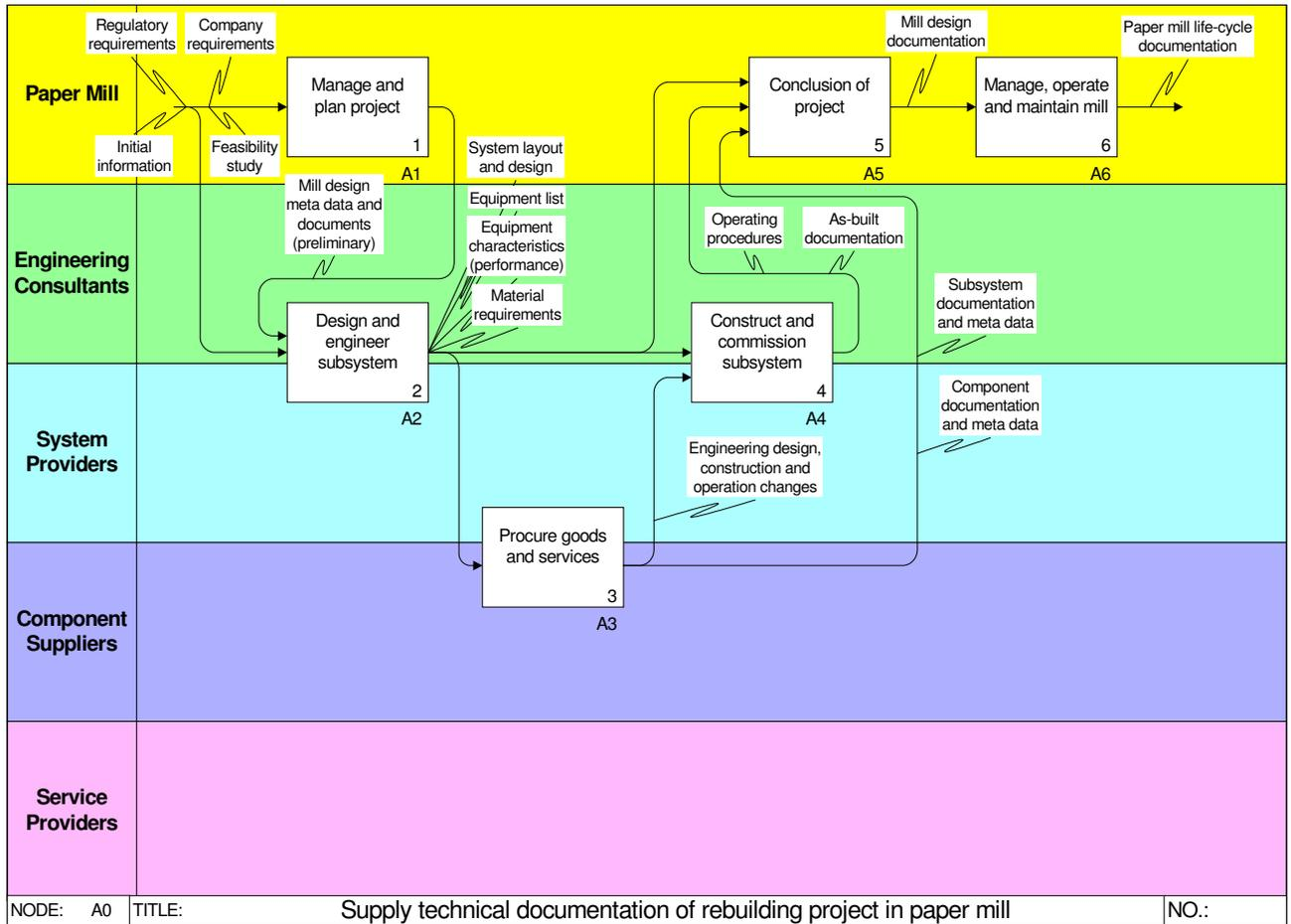
Figure 5. Main process diagram in the rebuilding of paper mill.
