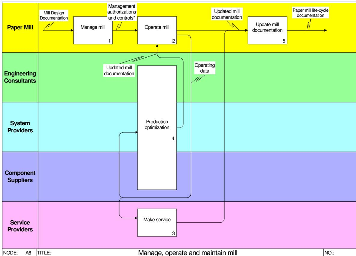
Figure 12. Manage, Operate and Maintain Mill.
