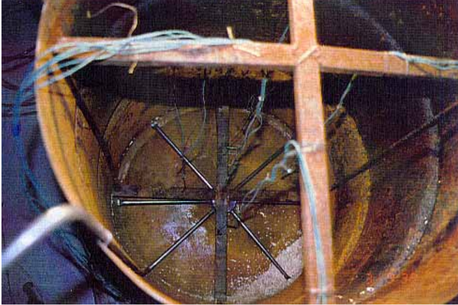
a) The gas feeding pipework on the bottom of the barrel. All other constructions belong to the thermocouple system.
