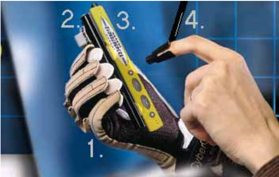
Figure 33. Real and virtual worlds combined. 1) Data glove, to simulate virtual hand and to accurately measure position and orientation of the user's hand and fingers. 2) Physical mock-up, where position and orientation can be measured with trackers. 3) Virtual prototype, which is overlapped with physical mock-up. 4) The Phantom haptic device.
