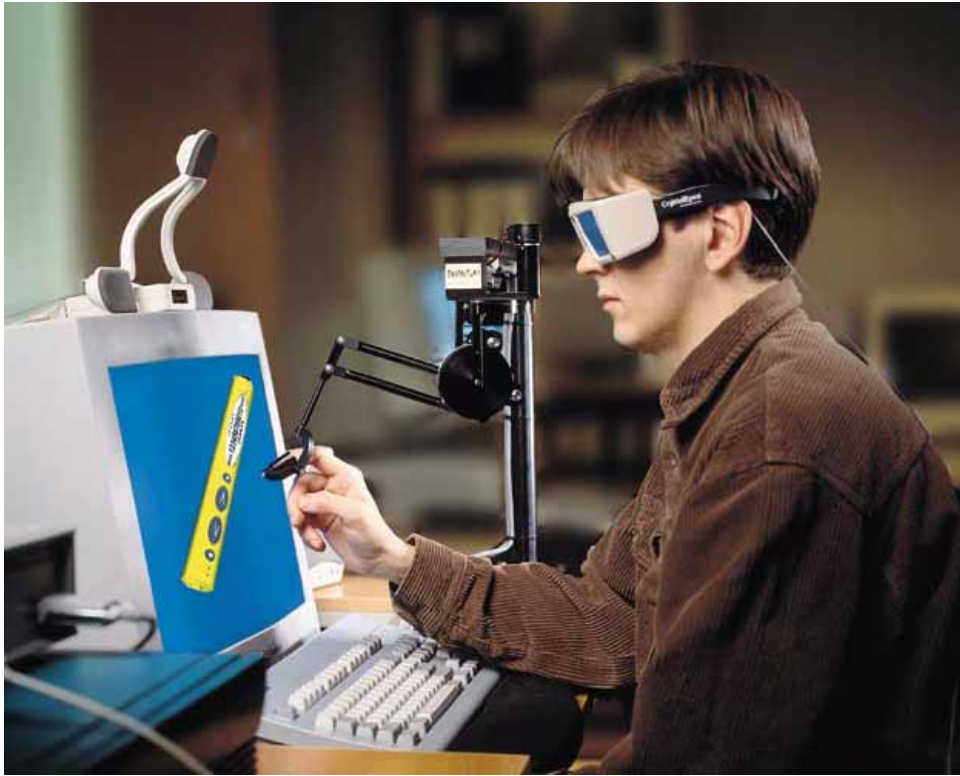
Figure 31. Virtual prototype's usability test with a haptic device.
