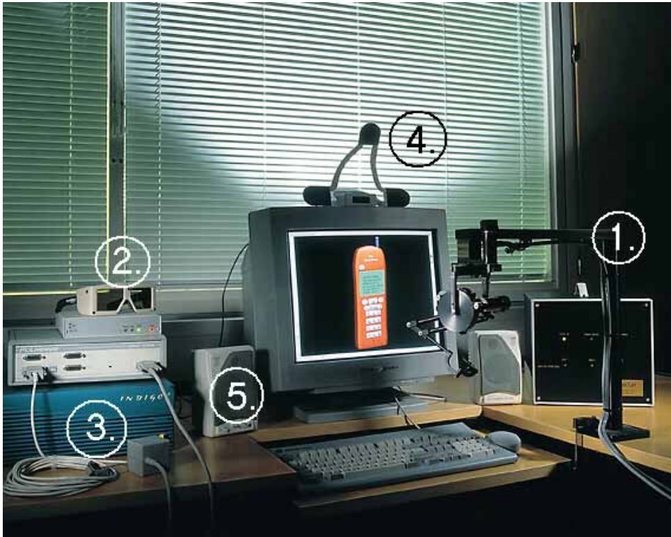
Figure 4. Virtual prototyping environment at VTT Electronics. 1) A haptic device, for receiving tactile and force feedback from virtual prototypes and for manipulating them by touch. 2) 3D glasses, to get a stereoscopic image of the simulated virtual prototype. 3) Efficient workstation, for haptic and visual rendering. 4) A head position tracker to find out the position of the head. When the user moves his/her head to look at the virtual prototype from the side, the visual scene changes so that it is possible to look at the object from different directions. 5) A soundcard with loudspeakers to output sound effects from the virtual prototypes.
