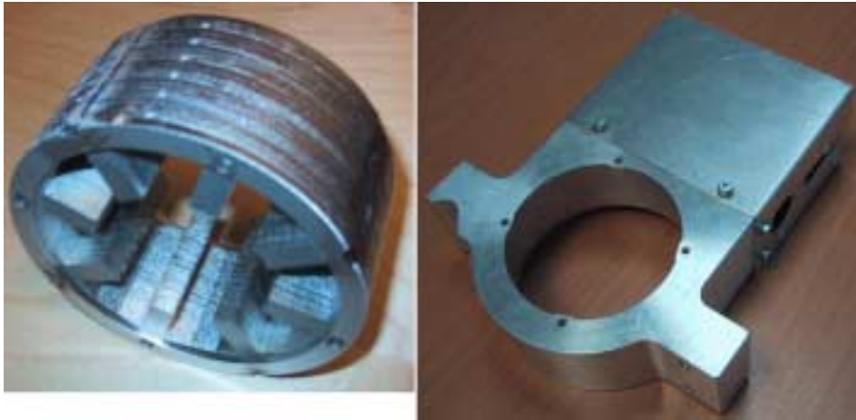
Figure 2. The actuator body (left) and the mount for the body (right). The read-out electronics and the cable connections were located in the aluminium box on the mount.
