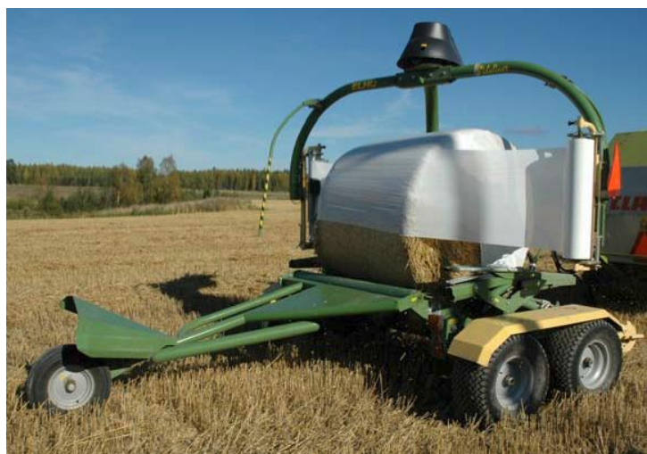
Fig. 2. Storage of chemically pretreated wheat straw in round bales. Wrapping of the bale with white stretch film.
