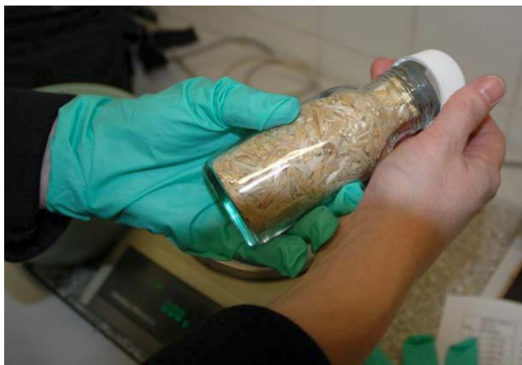
Fig. 3. Chemical storing of wheat straw in minisilos. Sealing with gray rubber plug and white plastic cap.
