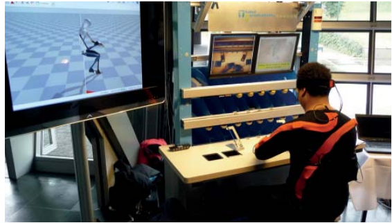
Ergonomics evaluation: automatic physical and cognitive load analysis, full body motion capture
