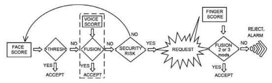
Fig. 1. Operation of a "three-stage" cascaded system (fusion with voice can be skipped if no voice data are available).
