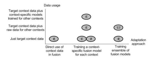
Figure 3: Choices of adaptation type and data usage in the four test cases: B – biometrics; R – recommender systems; E – emotion recognition; UI – interaction adaptation.
