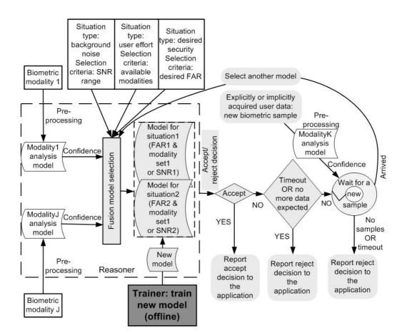
Figure 7: Lightweight adaptation for verification: grey colour indicates components developed for the multimodal fusion experiments.
