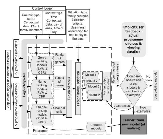
Figure 8: Adaptation of a TV recommender: the grey shading indicates components developed for the multimodal fusion experiments.
