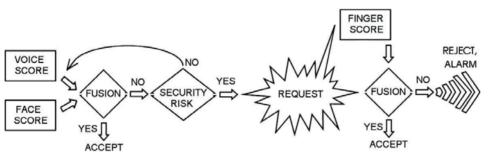
Fig. 2. Operation of a "two-stage" cascaded system.
