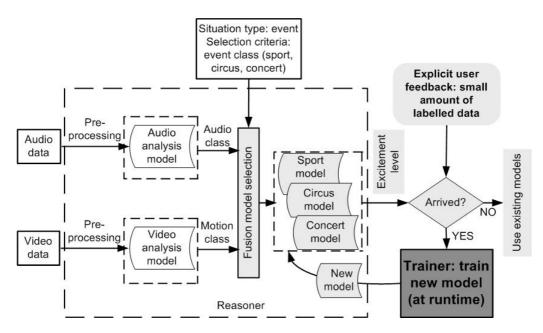
Figure 10: Adaptation for affect recognition: grey colour indicates components developed for multimodal fusion.
