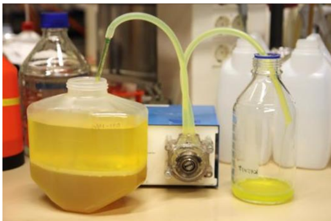
Figure 14. Phase separation by centrifugation after washing the surfactant phase with isobutanol. A “raft” is clearly visible between the two phases. The product (GFP-HFBI) was recovered in the lower aqueous phase by pumping.
