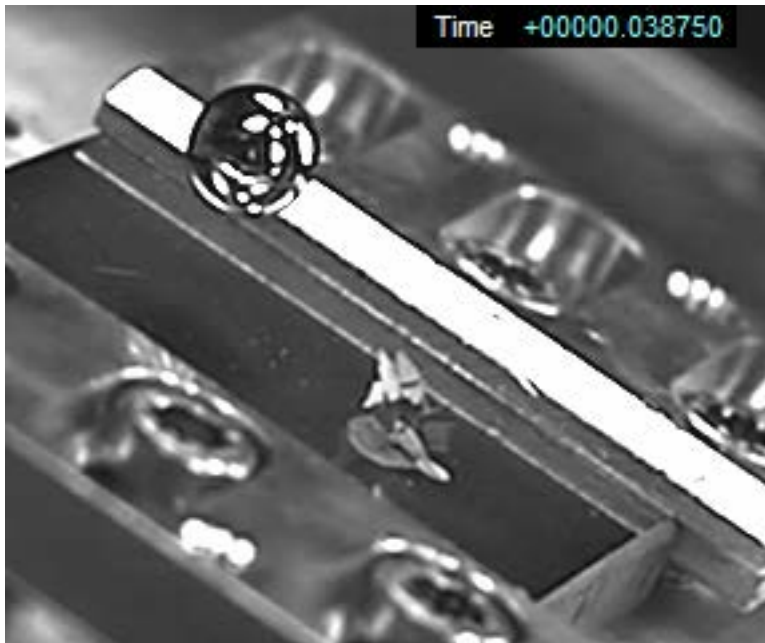
Figure 6.7: High speed video frame of an impact event showing the ejection of debris due to a compound impact sliding event for a spherical steel projectile against COMM3
