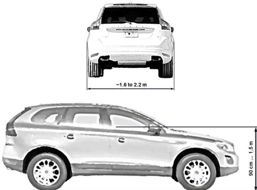
**Figure 17.** Vehicle width and height.
