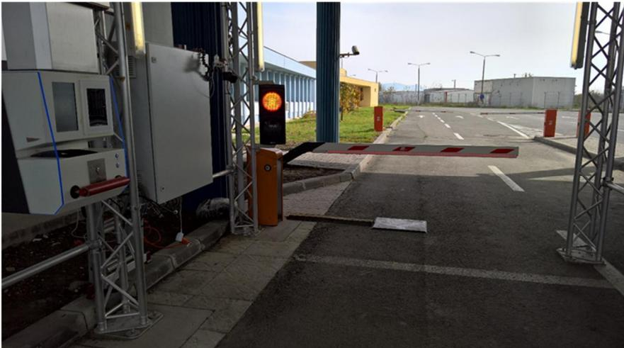
**Figure 28.** Acceptance tests were recorded with multiple synchronised cameras. The picture also shows the moving land border traveller terminals equipped with passport readers, cameras and intercom.
