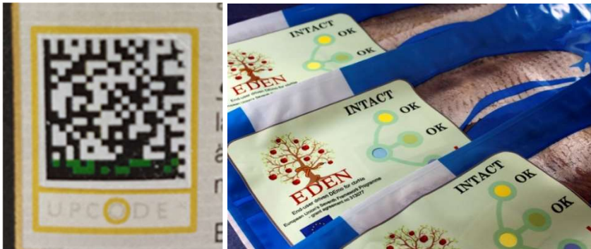
Figure 13. A 2D bar code with an integrated temperature sensing element (green bar), and visual indicators for oxygen to check package integrity.
