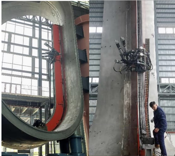
Figure 6.1. Robotic machine carrying out machining inside of the VV.
