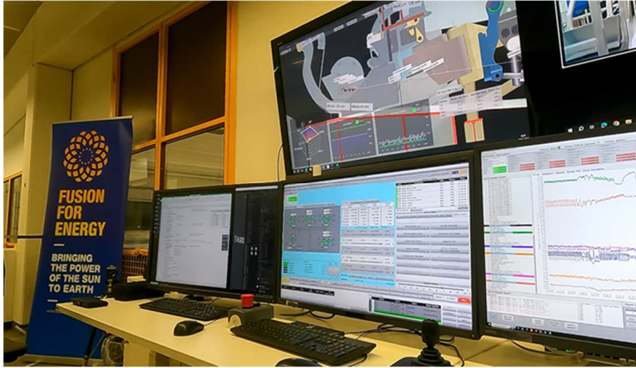
Figure 7.1. A view of the DTP2 operator room. The displays left to right; lower row: An Excel implementation of the Operations Management System, Command & Control operator user interface, and Remote Diagnostics Application; upper row: Virtual Reality, and camera view from the inner rail of the reactor towards the maintenance tunnel.
