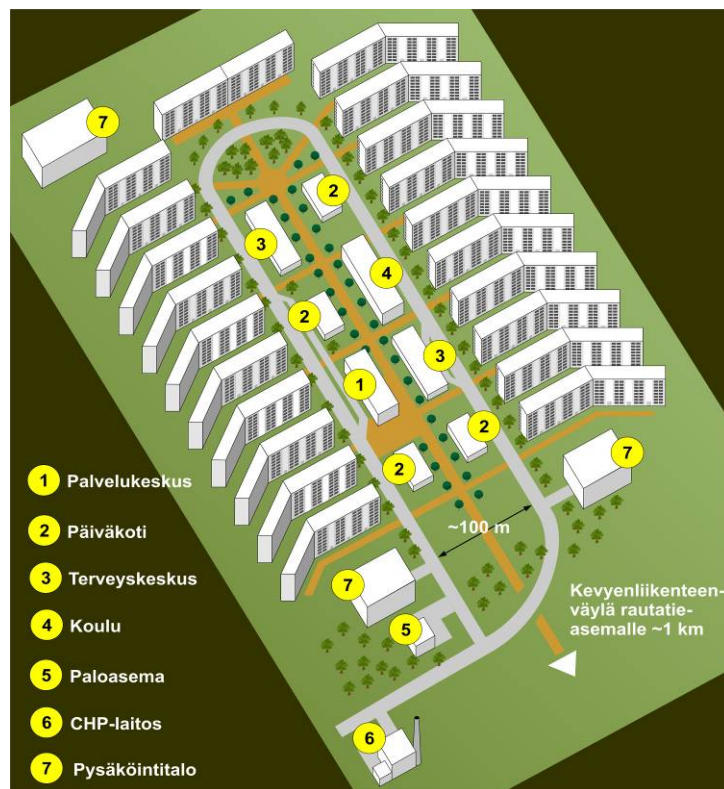
Figure 19. A layout showing the locations of high-rise residences, offices and consumer services. 1:service center, 2: day care, 3: health care center, 4: school, 5: fire station, 6: CHP plant, 7:parking house.
