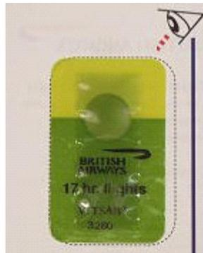
*Figure 3-3. Enzymatic time-temperature indicator (VITSAB).*
