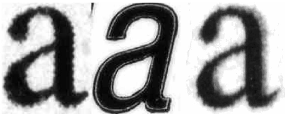
Figure 5-9. Rotogravure, flexography and ink jet printed letters.
