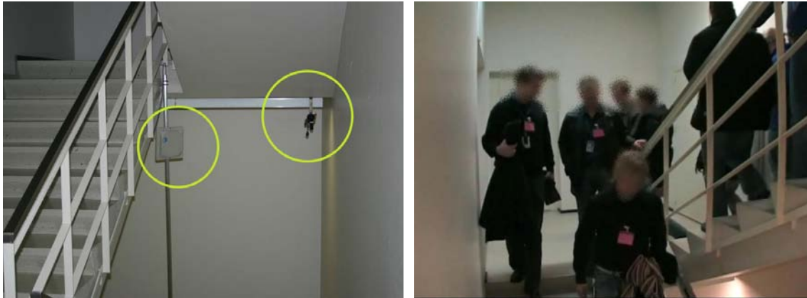
Figure 9. Left side: monitoring equipments between floor levels (RFID-antenna and DV-camera). Right side: snapshot of the DV-camera during the evacuation exercise, where also the (red) RFID-tags are shown. The RFID tag recognition region of the antenna was close to the first descending person in figure on the right side.
