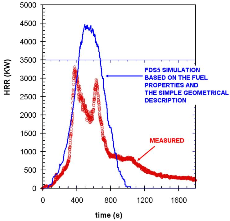
Figure 47. Comparison of the measured and simulated heat release rates of the office workstation fire experiment carried out by Madrzykowski and Walton [57].
