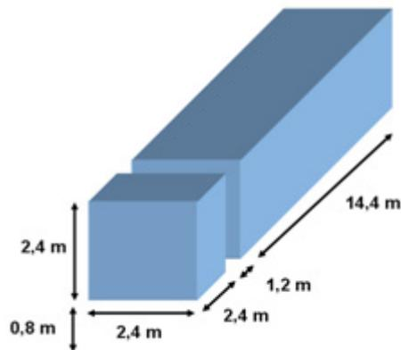
Figure 25. Estimate for HGV fire HRR corresponding to 95 % fractiles of the maximum HRR (50 MW) and fire load (245 GJ). The parameter values are:  $t_g = 60$  s,  $t_1 = 424$  s,  $t_2 = 3\,600$  s,  $\tau = 1\,600$  s. b) Simplified description of a burning HGV for the FDS fire simulation program (dimensions selected to fit e.g. a 20 cm or 40 cm computation mesh).
