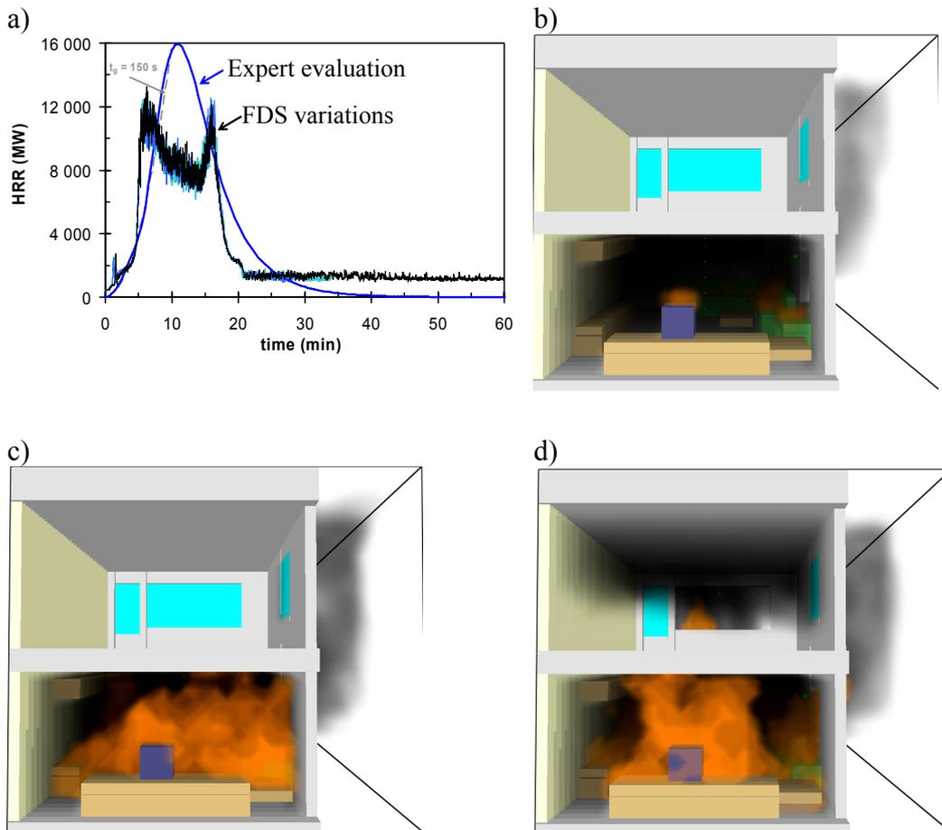
Figure 12. a) Comparison of two different approaches for determining heat release rate. An example of fire development in an apartment is shown in b)–d).
