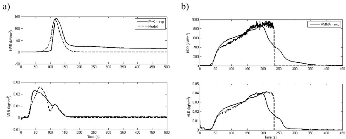
Figure 31. Examples of FDS5 predictions of small-scale fire experiment data (the cone calorimeter) on the basis of the material reaction kinetics: a) PVC and b) PMMA [55].
