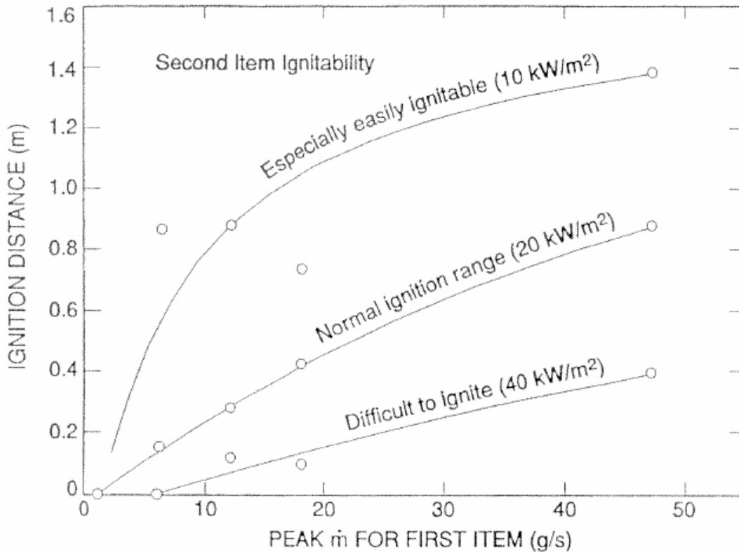
Figure 6. Relationship between peak mass loss rate and ignition distance for various ignitability levels (radiant flux) [8, 9].
