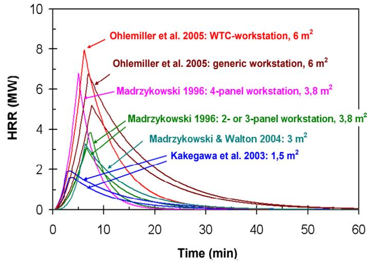
Figure 3. Data from fire experiments with office workstations [3, 4, 5, 6].
