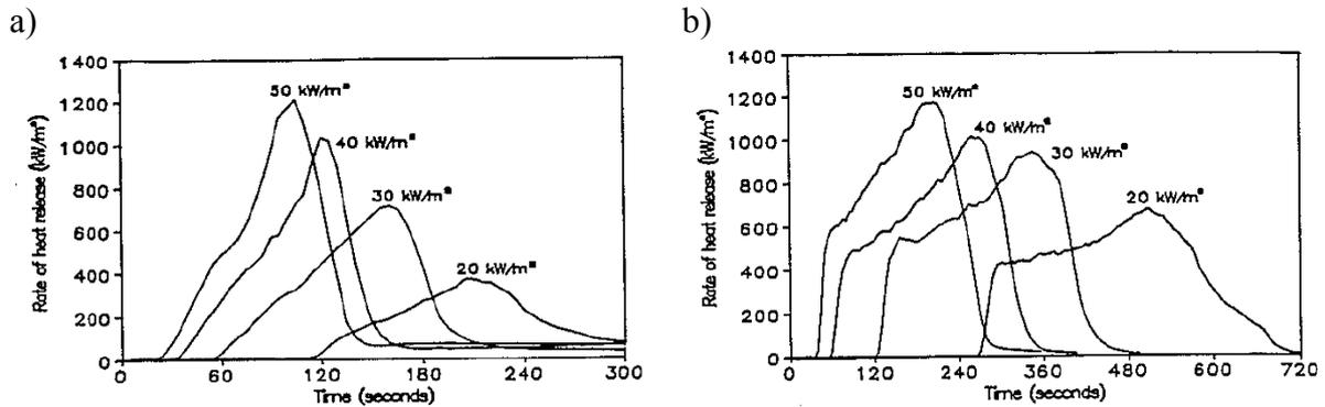
Figure 37. Examples of the influence of the cone calorimeter heat flux on the measured HRRPUA: a) PP and b) ABS. Data from [61].
