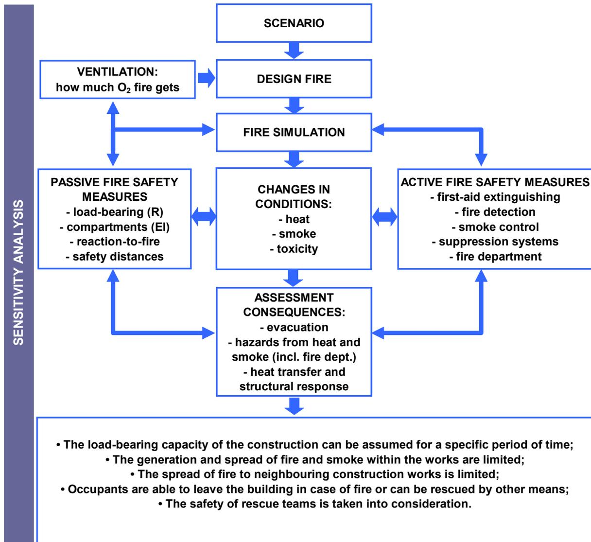
Figure 2. Fire safety engineering analysis scheme.
