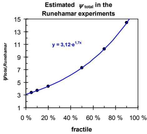
Figure 23. Estimated fractiles of the total enhancement factor  $\psi_{total}$  in the Runehamar experiments.
