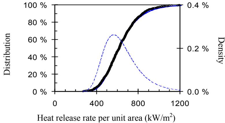
Figure 14. Intensity of fire in a living room. The distribution shows how much heat is released per floor area (average 640 kW/m<sup>2</sup>, 80 % fractile 770 kW/m<sup>2</sup>).
