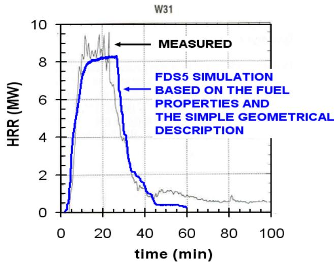
Figure 42. Comparison of the measured and simulated heat release rates of the EUREKA fire experiment W31 [78].
