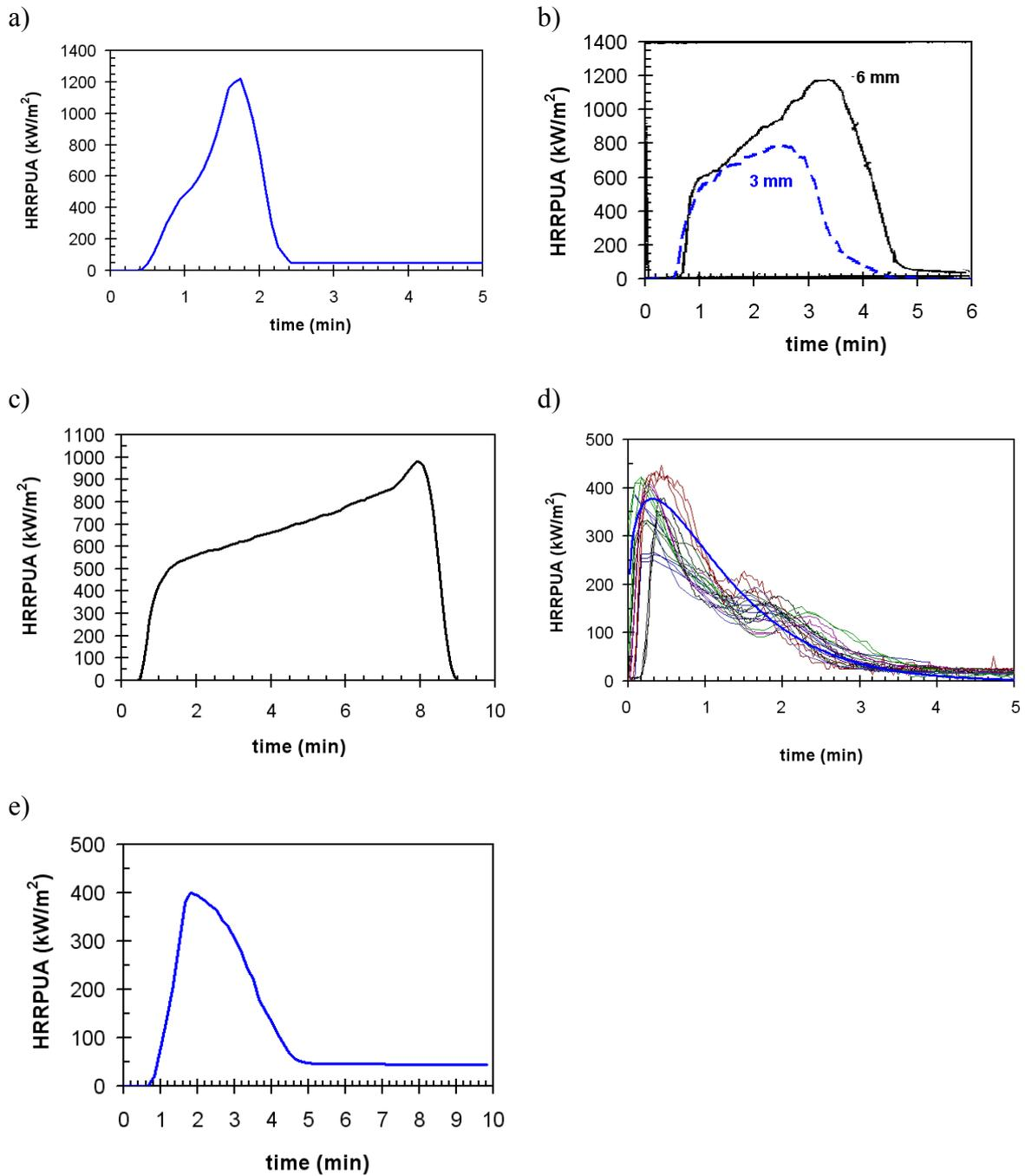
Figure 36. Examples of cone calorimeter data on paper/cardboard samples at heat exposure of 50 kW/m<sup>2</sup>: a) 3 mm thick PP, b) ABS: the dotted curve is a 33-g or about 3-mm plastic sample from a washing machine [60] and the solid curve data from [61], c) black PMMA (plexiglass), 12 mm [62], d) flexible PU foam studied in the SAFIR project Round Robin exercise [63] and e) PET [64].
