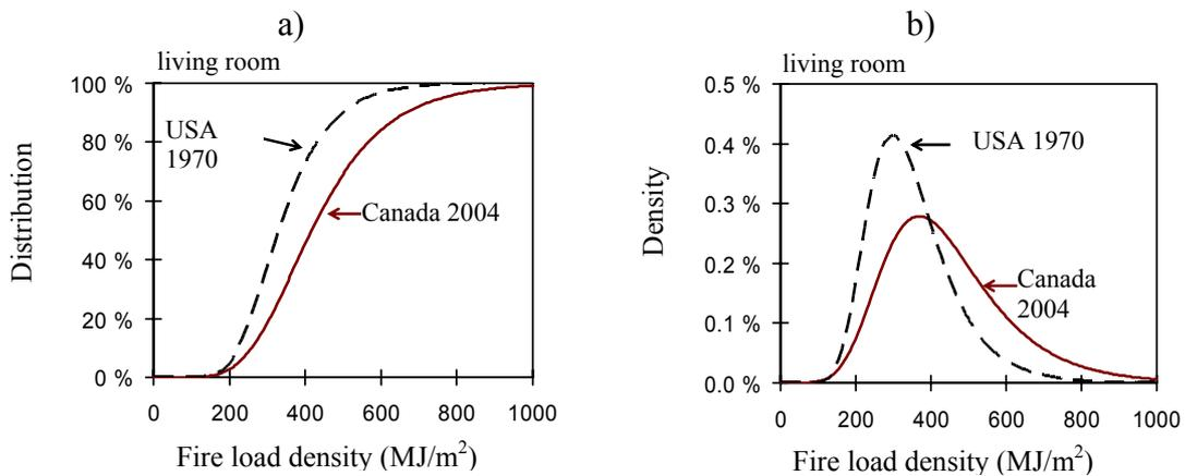
Figure 10. Fire load density in living rooms in Canada 2004 with comparison to a congruous study in USA 1970: a) cumulative distribution function and b) density function.
