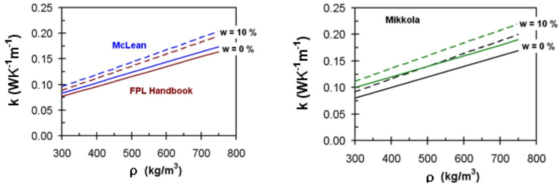
Figure 39. Dependence of the thermal conductivity of wood on its density at room temperature at moisture contents of 0 % and 10 %.
