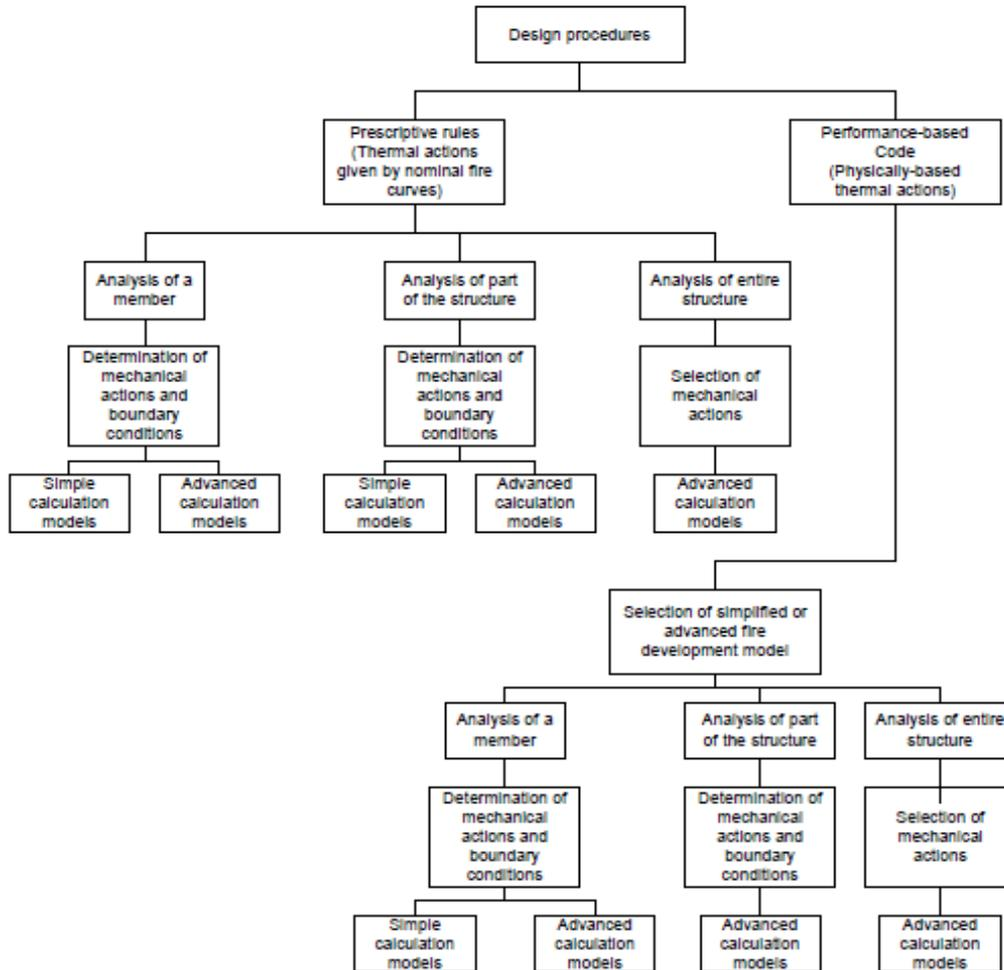
Figure 48. Design procedures according to EN 1995-1-2.
