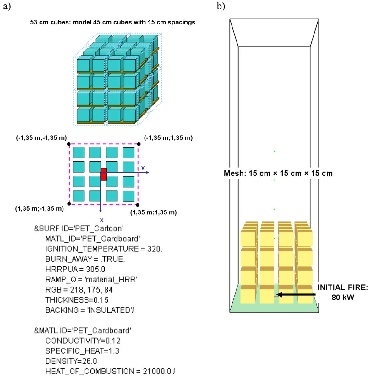
Figure 44. The FDS5 model of PET/cardboard fire experiment: a) schematic description and b) the actual model.
