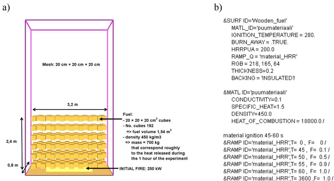
Figure 41. a) FDS5 model of the EUREKA fire experiment W31 and b) model parameters.
