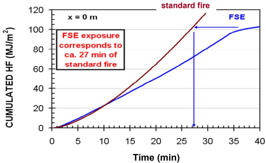
Figure 52. Integrated heat fluxes of standard fire and FSE heat fluxes of Figure 51.
