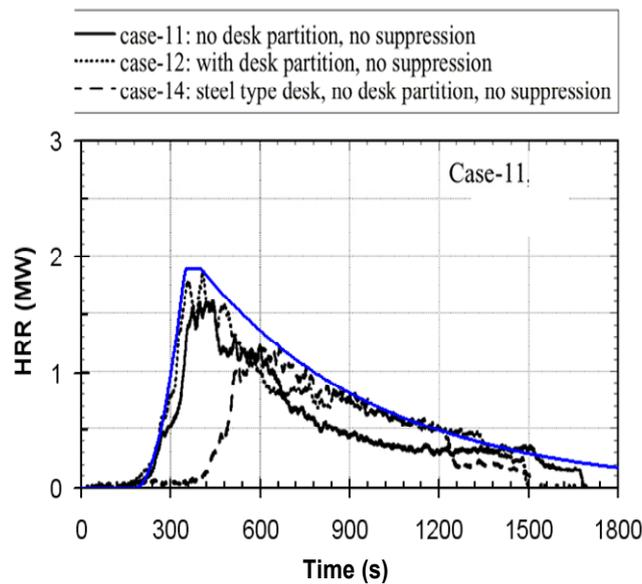
Figure 4. Example of modelling of experimental HRR data by a simplified model.
