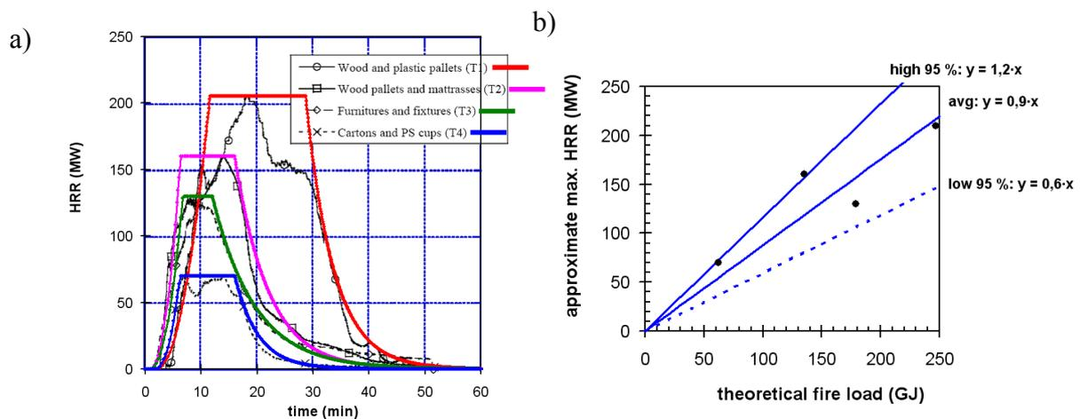
Figure 19. HRR results of Runehammar experiments [46]. The coloured curves represent  $t^2$ -models that reproduce the growth and decay phases as well as the peak HRR with reasonable accuracy (adjustment of the curves to fit the data is done only visually by the author of this document). b) Display of the apparent correlation ( $R^2 = 0.97$ ) between the fire load of the burned item and the maximum HRR.
