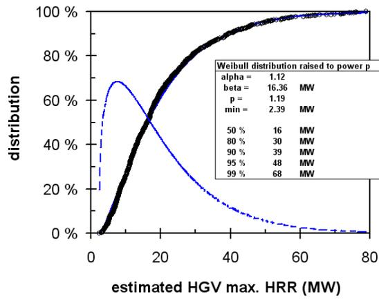
Figure 24. Estimate for the distribution of the HGV maximum heat release rate.
