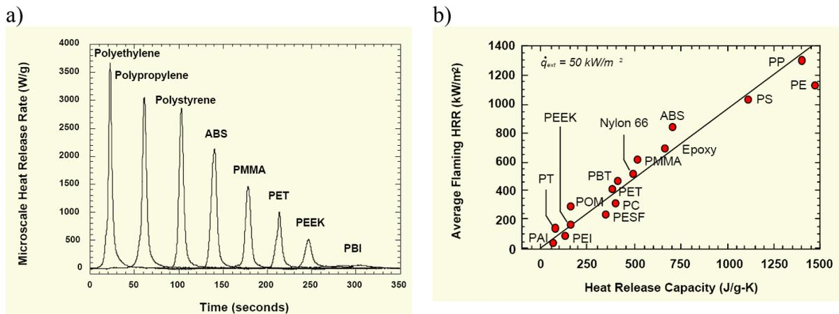
Figure 35. Examples of combustibility ranking of plastics given by Lyon & Walters [58]: a) TGA/DTA data and b) HRRPUA vs. the heat release capacity of the material.
