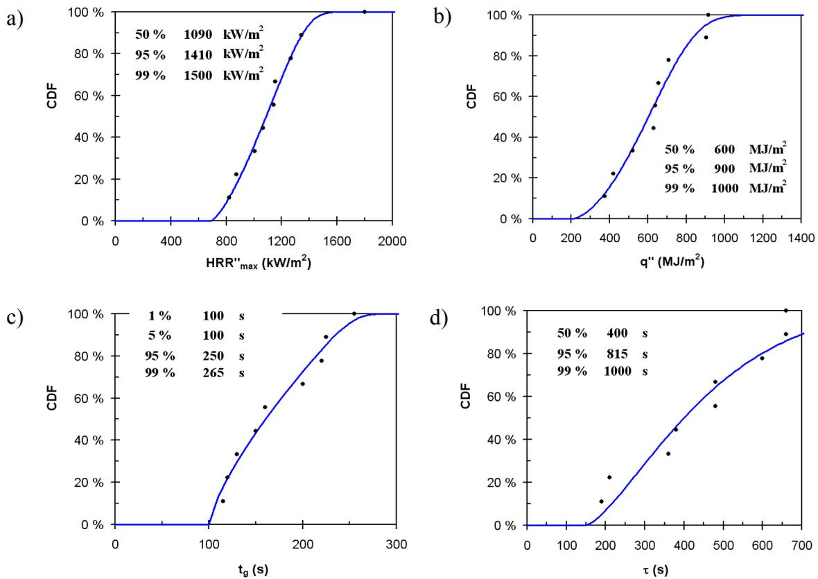
Figure 5. Example of statistical analysis of office workstations: a) HRR/m<sup>2</sup>, b) total heat release/m<sup>2</sup>, c) HRR growth time factor t<sub>g</sub> and d) HRR decay factor τ. (CDF = cumulative density function).
