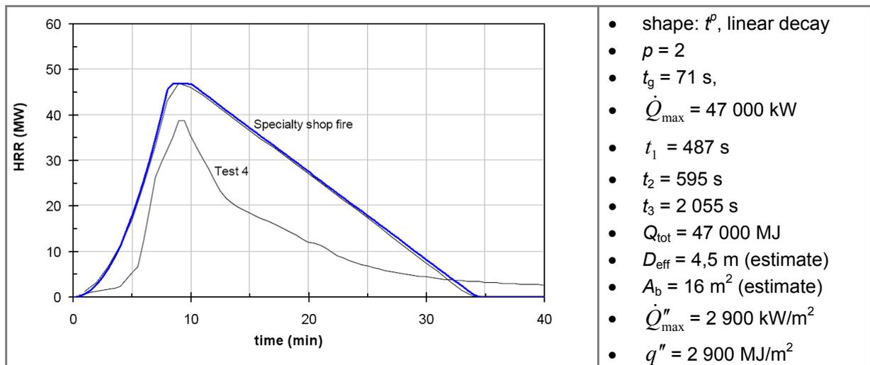
Figure 27. Heat release rate of a flashover fire in a specialty shop [51].
