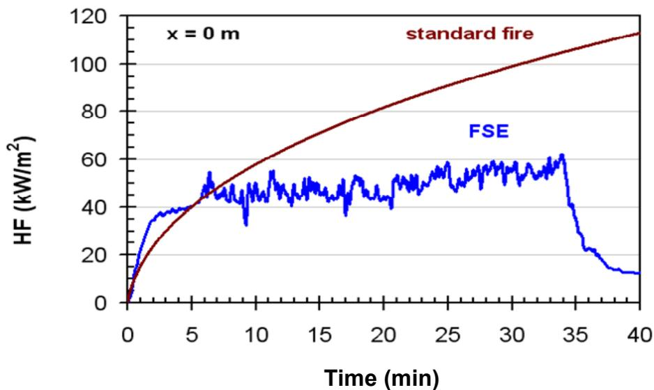
Figure 51. Heat fluxes of standard fire curve and FSE curve of Figure 50.
