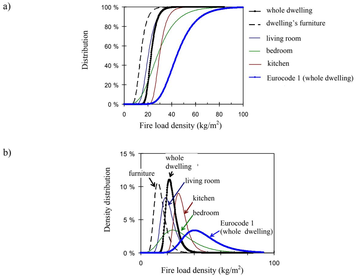
Figure 7. Comparison between results on block of dwellings fire load density distribution from Holm and Oksanen [16], a study published in 1970, and Eurocode 1 [17]. Units presented in a) cumulative distribution function and b) density function are  $\text{kg}$  dried wood per floor area ( $\text{m}^2$ ).
