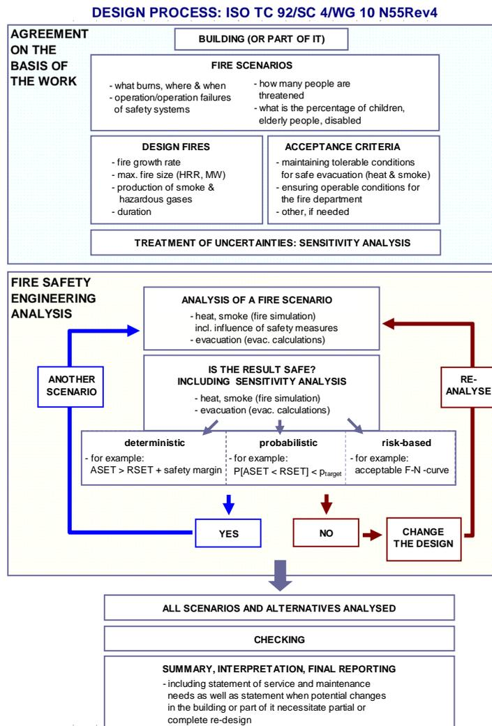
Figure 1. The FSE design process scheme.
