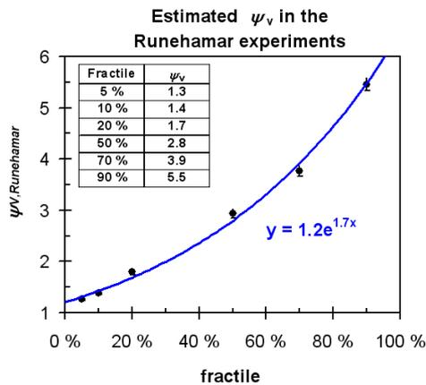
Figure 22. Estimated fractiles of the ventilation enhancement factor  $\psi_v$  in the Runehammar experiments.
