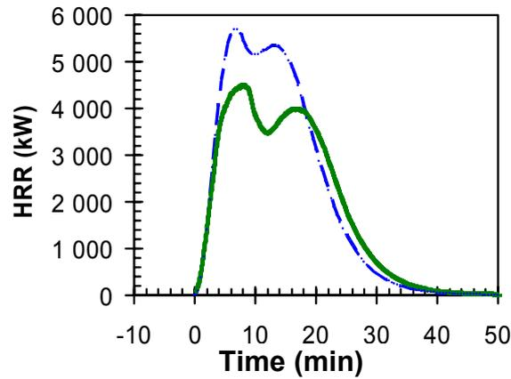
Figure 17. Modelled curves based on the results of room fire experiments by Blomqvist et al. [43]: the heat release rate curve using methodology explained above for open space fire (dashed line) and for oxygen restricted fire (solid line).
