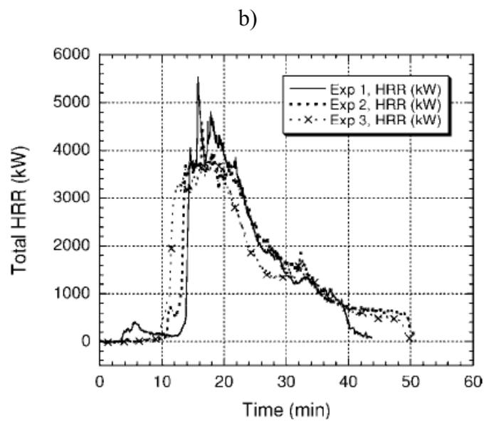
Figure 16. a) Furniture setting in the room fire experiment series performed by Blomqvist et al. [43], and b) the measured heat release rates.
