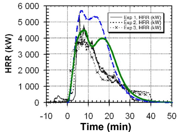
Figure 18. Comparison of heat release rates measured in the room fire tests (Blomqvist et al. [43]) and calculated using the presented model.
