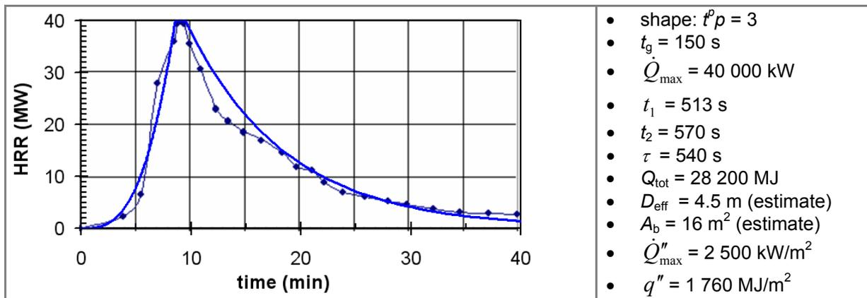
Figure 26. Heat release rate of a flashover fire in a shoe storage room [51].
