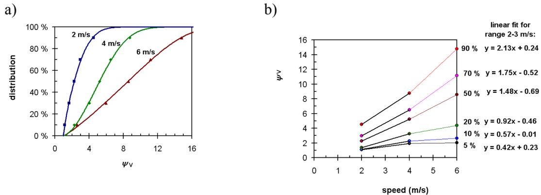
Figure 21. a) Estimated distributions of  $\psi_v$  for flow speeds based on the fractiles presented by Carvel et al. [49] and b) 5–90 % fractiles of  $\psi_v$  vs. the flow speed.
