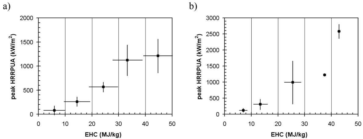
Figure 34. Examples of cone calorimeter fire experiment data on plastics at heat exposure of a) 40 kW/m<sup>2</sup> and b) 70 kW/m<sup>2</sup>. Data taken from [59] and averaged over five EHC classes: EHC < 10 MJ/kg, 10 MJ/kg ≤ EHC < 20 MJ/kg, 20 MJ/kg ≤ EHC < 30 MJ/kg, 30 MJ/kg ≤ EHC < 40 MJ/kg and EHC ≥ 40 MJ/kg.
