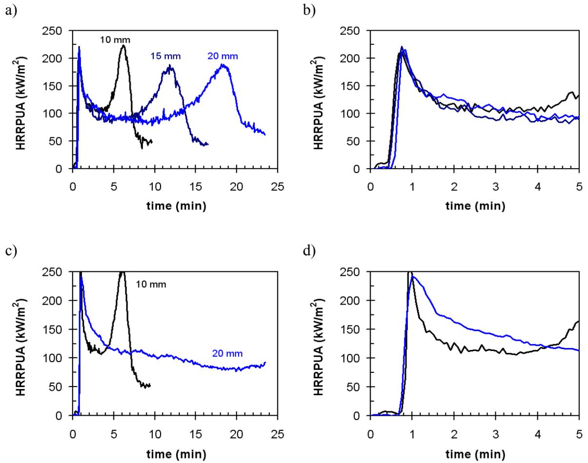
Figure 32. Examples of cone calorimeter data on wooden samples at heat exposure of 50 kW/m<sup>2</sup>: a) and b) Finnish pine with three thicknesses (b shows the first 5 minutes of the experiment), and c) and d) Finnish spruce with two thicknesses (d shows the first 5 minutes of the experiment) [56].
