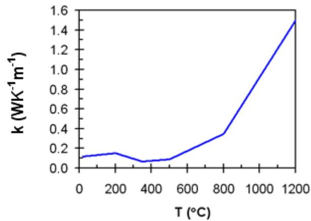
Figure 40. Temperature dependence of thermal conductivity of wood according to EN 1995-1-2.
