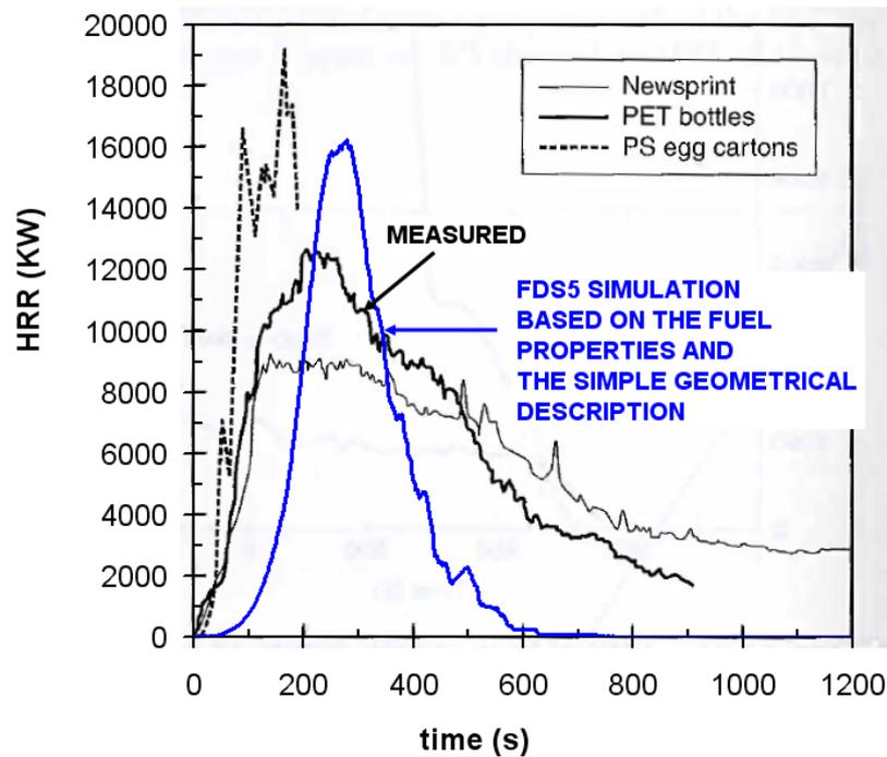
Figure 45. Comparison of the measured and simulated heat release rate of fire experiment on PET plastic bottles in cardboard boxes.
