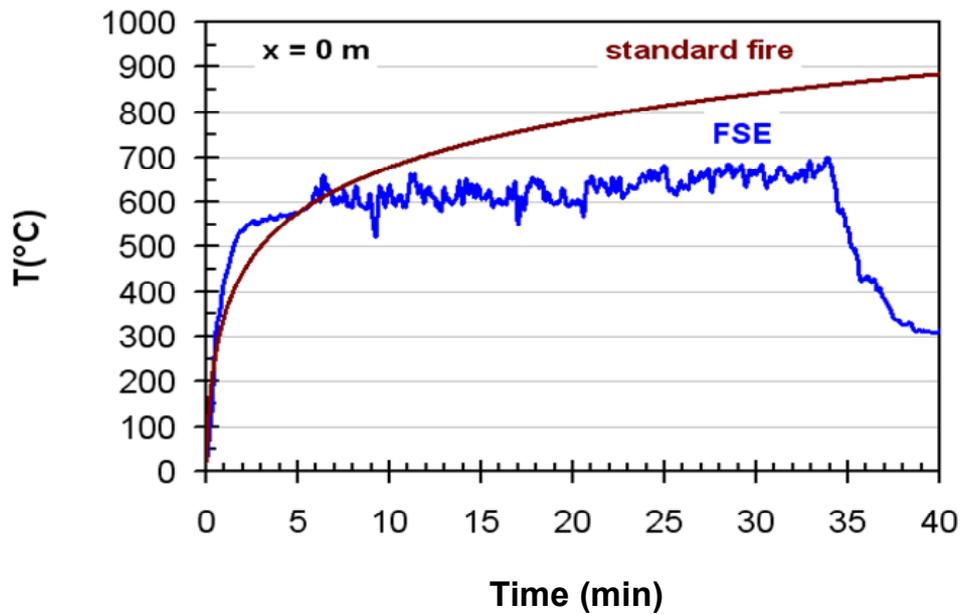
Figure 50. Standard fire curve and an example of a design fire curve (FSE).
