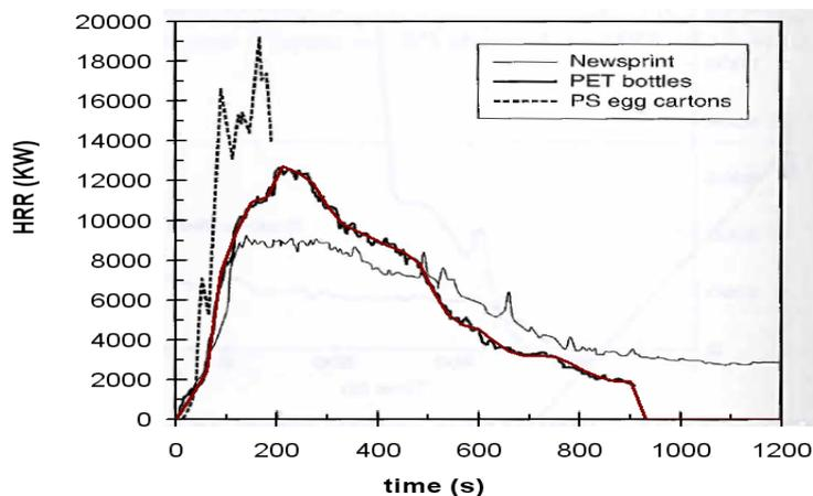
Figure 43. Heat release rate measured in the fire experiment with PET plastic bottles in cardboard boxes. Reproduced from [79].
