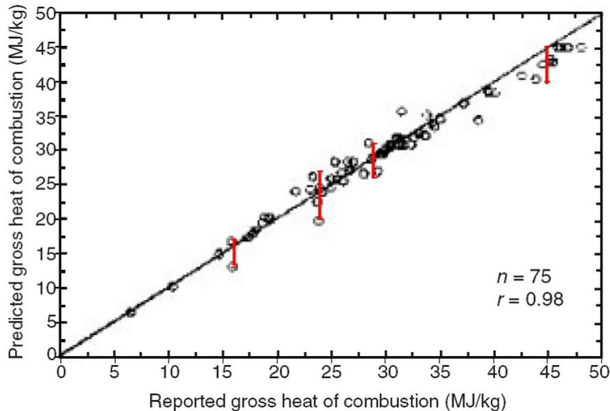
Figure 38. Example of the heat-of-combustion prediction developed by Hshieh et al. [65] for pure organic polymers.
