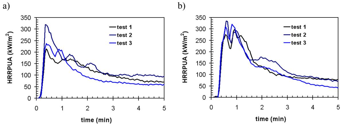
Figure 33. Examples of cone calorimeter data on paper/cardboard samples at heat exposure of 35 kW/m<sup>2</sup>: a) about 400 g of paper stacked dwelling and b) paper stacked dwelling covered with cardboard. Data from [57].
