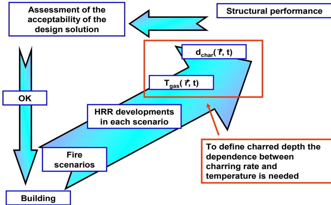
Figure 49. Design concept for structural performance of timber.
