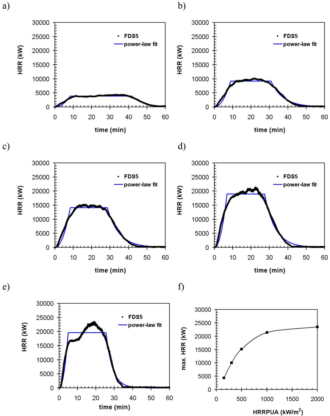
Figure 30. Evolution of the shelf system HRR for different fire load HRRPUA values: a) 150 kW/m<sup>2</sup>, b) 300 kW/m<sup>2</sup>, c) 500 kW/m<sup>2</sup>, d) 1 000 kW/m<sup>2</sup>, e) 2 000 kW/m<sup>2</sup> and f) maximum HRR vs. HRRPUA. The blue curves in a-e show t<sup>2</sup>-shaped fits to FDS results.
